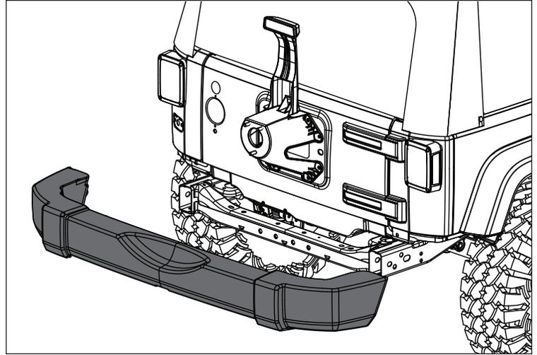
2. Align left and right mounting brackets into frame rail.
