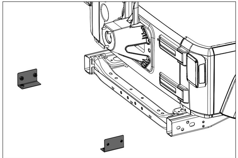
3. Align rear bumper with body. Using supplied M14 hardware, attach rear bumper to vehicle.
