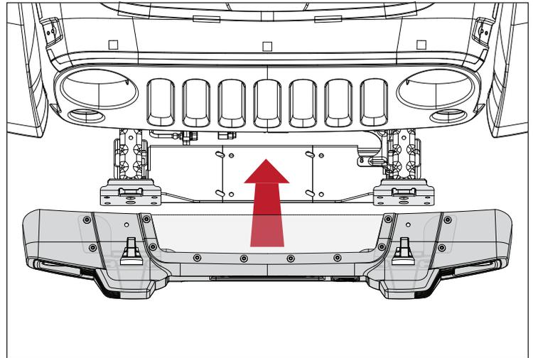
28. Place Stanchion, Bumper Mount Bracket, and factory Tow Hook on frame horns and secure with OE Nuts. If not using Tow Hooks, replace with M12 Hex Head Bolts and Lock Nuts.
