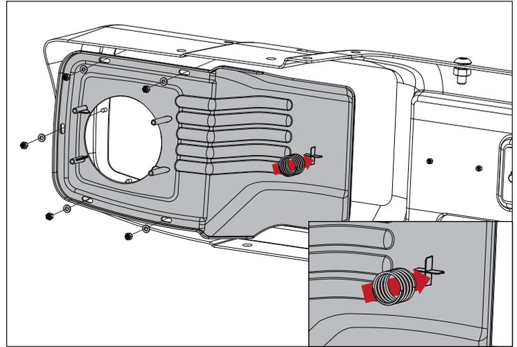
4. Remove bulb from factory fog light housing and install housing to bosses in Plastic Cover using supplied Thread Forming Screws. Do not overtighten.
