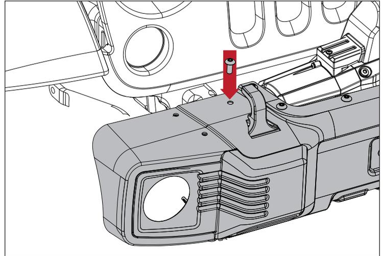
35. Install Bumper Ends, aligning mounting points of Bumper Ends, Center Section, and Mounting Bracket, using supplied M10 Button Head Bolts and Plastic Flat Washers.
