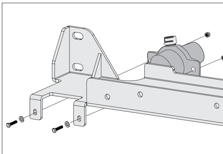
17. Install Winch Plate by first placing Bottom Plate between frame horns.
