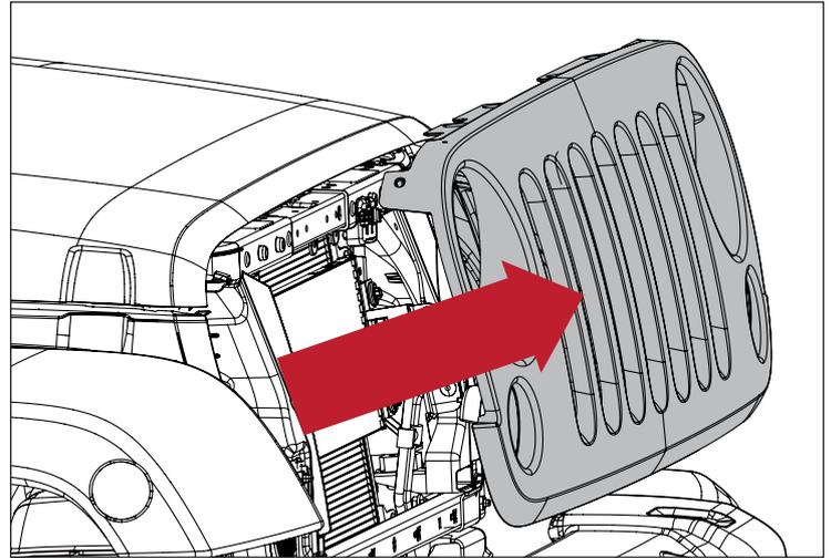
11. Remove factory plastic closeout panel by releasing the plastic fasteners that attach it to each frame rail.
