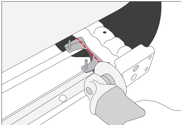
15. Disconnect hose retainer clips from vacuum pump and remove zip ties holding air lines.
