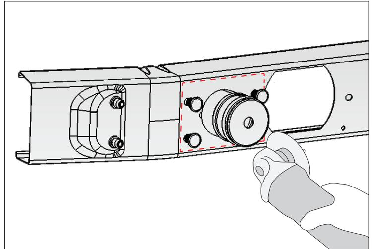
25. Insert Tow Hooks into opening in Bumper Center Section. If not using Tow Hooks, replace with M12 Hex Head Bolts. Place Crush Can and Bumper Mount Bracket in place in front of Tow Hooks or M12 Bolts.
