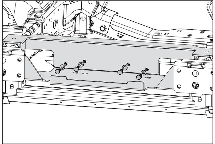
20. Attach Winch Plate to top of each frame horn using M10 Hex Bolt and M10 Nut Plate supplied with Winch Plate.
