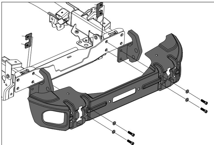
8. Loosely attach Light Bracket using supplied M12
