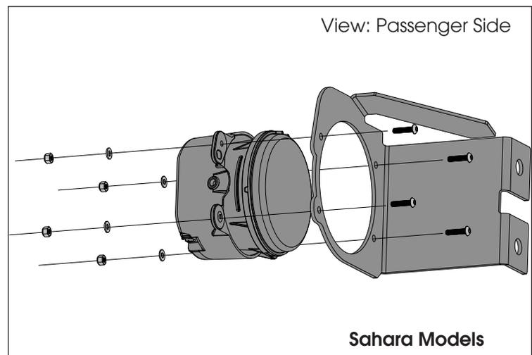
4. Remove OE Frame Horn Brackets. Reusing OE bolts from Frame Horn Brackets, loosely attach Winch Tray.
