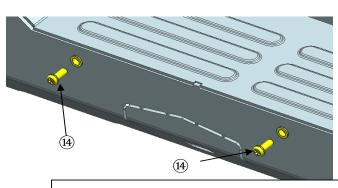
Block the hole where the license plate bracket was originally installed with a cross groove pan head screw
