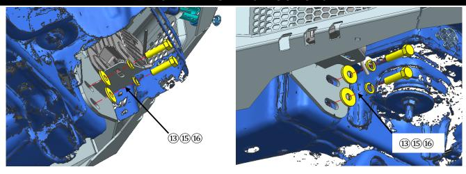
4.3 Adjust the gap between the rear bumper and the vehicle, plug the license plate light and radar harness plugs
