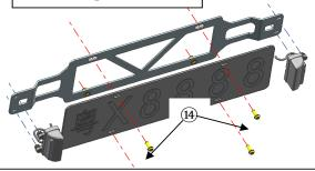
First, use (4) cross slot pan head screws to install the license plate onto the holes at the bottom of the license plate bracket
