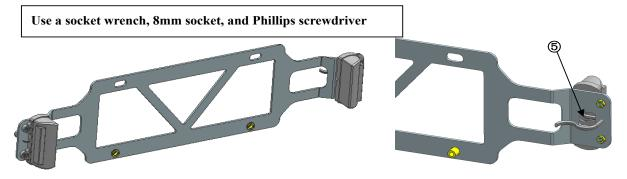
Install the license plate light onto the license plate bracket and the  $\ensuremath{\mathfrak{G}}$  through the license plate light hole
