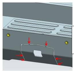
Cut off the cover on the bumper with an angle grinder and wrap it with a tape
