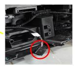
4.2 Push the plates on both sides of the rear bumper parallel to the vehicle bracket on both sides of the original beam, adjust and lock them.
