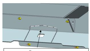
Connect the **®**license plate extension cable and insert it into the rear bumper through this square hole
