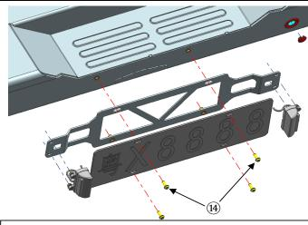
Check if the license plate extension cable has passed through the middle square hole. After passing through, use the remaining 4 cross slot pan head screws to install the license plate and license plate bracket onto the bumper.
