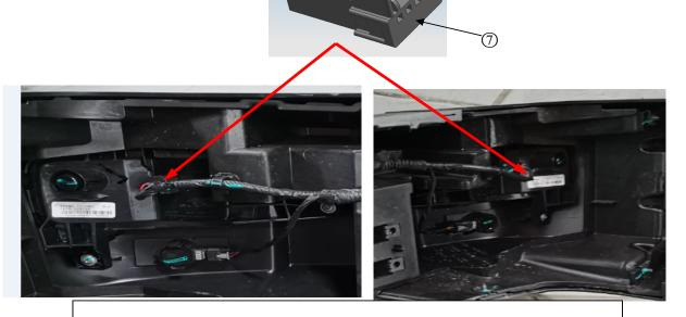
Insert ⑦ Fog Light Plug(Waterproof) x2 into the left and right fog light of the wiring
