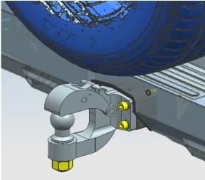
Install the trailer hitch onto the vehicle
