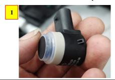
Remove the transparent plastic pad from the radar
