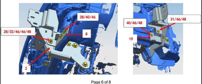
Step 4.2 Install the Winch frame connector as shown below.
