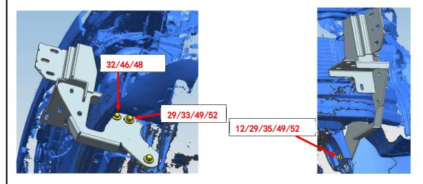
Step 4.1 Assemble support brackets on winch frame, please repeat above steps to right hand side.
