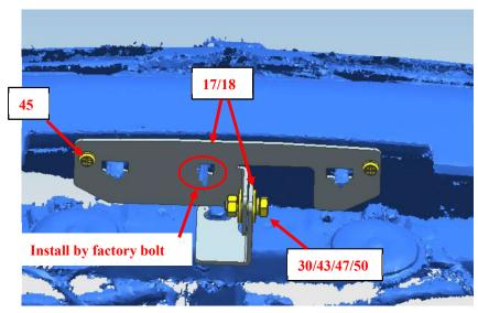
Step 3 Install the winch frame bracket and install it in the corresponding position of the body by hardware 23891011 as shown below, please repeat above steps to right hand side
