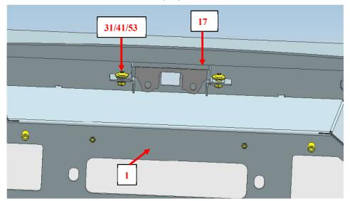
Step 6 Assemble bumper assembly and winch bracket by hardware as shown below.
