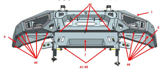
Step 8 Assemble the licenses bracket 16 18 on the bumper by 16 18 37 44 47 52
