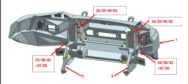
Step 7 Assemble the skid plate (5)(6)(7) to the bumper by (4)(4)(4).
