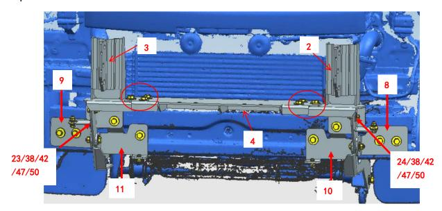
Step 5 Install camera holder on the bull bar body by hardware as shown below.
