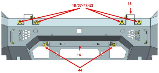
Step 9 Test and make sure that the guard is steadily fixed, fully tighten all hardware.
