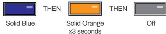
If a Factory reset was done on the Cabin module, the LED behavior is the following:
