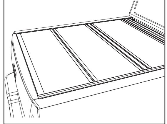
**OPENING COVER:** Lower the tailgate and pull the cable on either side. While pulling on the cable lift the panel up and towards the cab.
