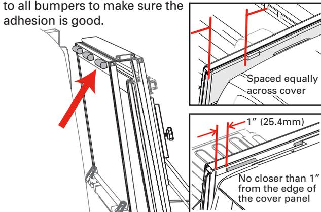
**12** Unfold the cover (C) towards the tailgate. Then confirm each panel is centered side to side and front to back on the truck bed. If adjustments are needed, loosen the cover retainer clamps (F) and shift the cover until positioned correctly. The rear edge of the cover and tailgate seal should rest on top of the tailgate. For proper sealing, the tail panel will overlap by .5".
