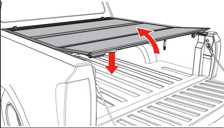
**FOLDED UP POSITION:** To drive with the cover (C) in the folded up position, use the straps and buckles provided with the cover. Attach the buckle at the bulkhead, then pull the strap to take up the slack and secure the cover.
