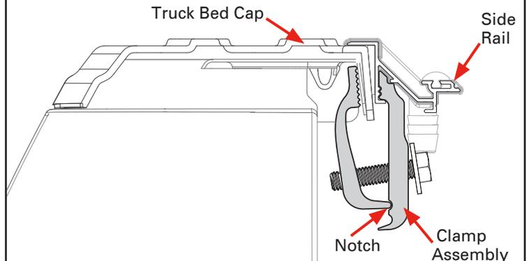
**7** Before placing the cover (C) onto the vehicle, slide two cover retainer clamps (F) into the track on the underside of the cover (C) near the cab. Confirm the cover retainer clamps fit properly into the cover rail for optimum fit. Repeat on the opposite side of the cover.
