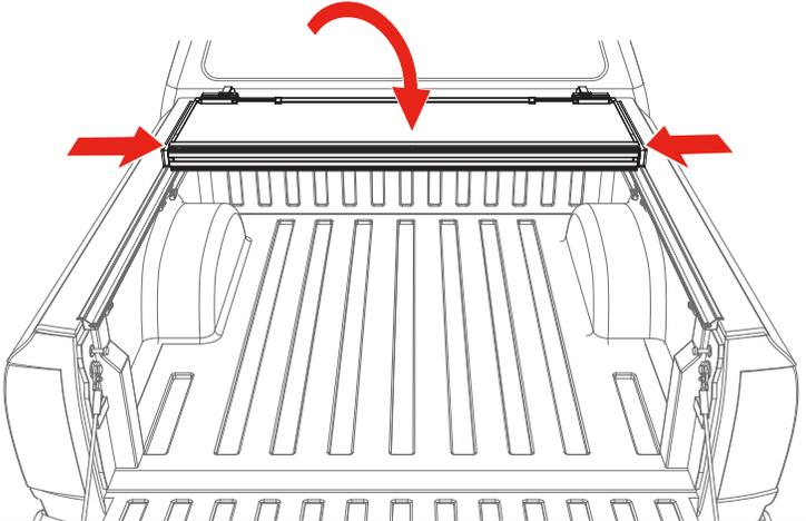
**10** Confirm the retainer clamps (F) are positioned around the side rails (A & B) correctly as shown below. Tighten the retainer clamps by turning them clockwise until the lock washer is secure.
