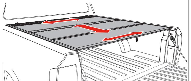
**13** Check if the latches are hitting or not engaging the side rails (A & B) by releasing each latch. If any of the latches need modifications refer to the Slam Latch Adjustment section on the next page on how to make adjustments.
