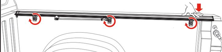
**NOTE:** If the rails are leaning down, have one person stand on the outside of the bed and slightly roll the rails upward while another person slowly snugs the clamps up. If the clamps are tightened too quickly or overtightened, it will cause the rails to lean down.
