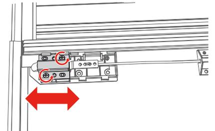
With the latch cover removed, loosen the screws and move the latch bracket to adjust. Retighten the screws. Slide the latch housing back on.
