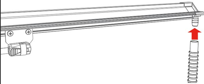
**4** Place the passenger side rail (A) on the truck rail. Position the side rail flush with the top edge of your truck bed rail. The end of the side rail with the drain tube will go towards the cab of the truck.
