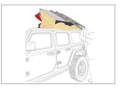
9. Allow the ladder to rest on the ground. If the ladder is extended too far it will need to be adjusted. (See next step) The ladder should be at a slight angle so it can support the tent while open.
