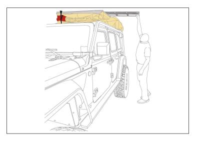
8. Use the ladder as leverage to open the tent, carefully folding it to the open position.
