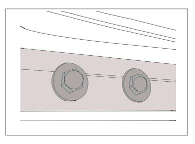
3. Mount the ladder brackets to the ladder using the supplied M6 bolts, washers, plastic washers, and nut. Plastic washers will go on both sides of the bracket on the ladder. **Do not over tighten bolts, there should be a slight resistance when rotating the ladder.**
