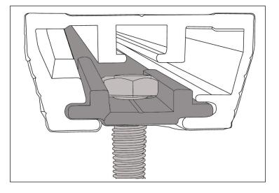
5. Secure the rooftop tent to your roof rack or roof bars. Use 2 M8 bolts and 2 slide plates with the base plate to secure the bar. If the cross bars are too far apart the center will not be properly supported and may be damaged.
