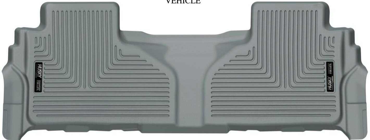
TO EASE INSTALLATION OF SECOND SEAT LINER, MOVE BOTH FRONT ROW SEATS TO THEIR MOST FORWARD. WITH THIS DONE, INSTALL YOUR LINER, POSITIONING IT AS SHOWN IN THE IMAGE ABOVE. ONCE THE LINER IS INSTALLED, REPOSITION THE FRONT SEATS AS DESIRED.
