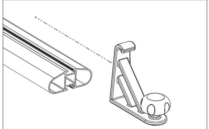
2. Tighten the twist knob until the Load Stops do not move and are locked in place.
