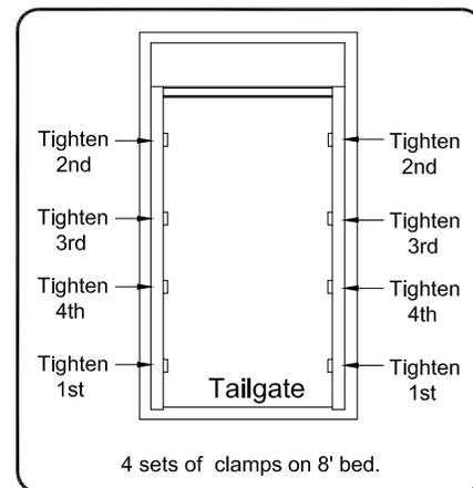
Tighten bed clamps to the track clamps. Note: When tight there may be a gap between the clamps, do not overtighten.
