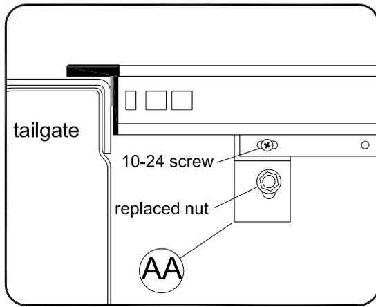
With track correctly back against tailgate tighten 10-24 screw. Adjust track to correct height and tighten nut.
