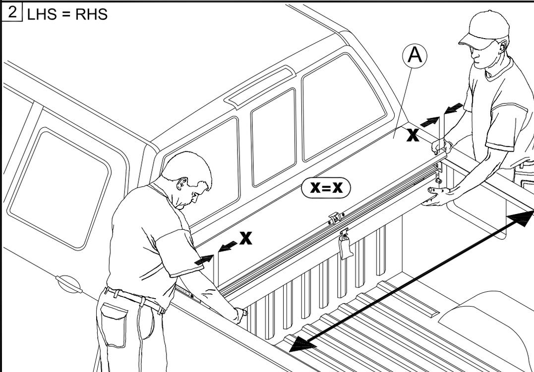
Center the Housing **A** between the bed rails up against the bulkhead.
