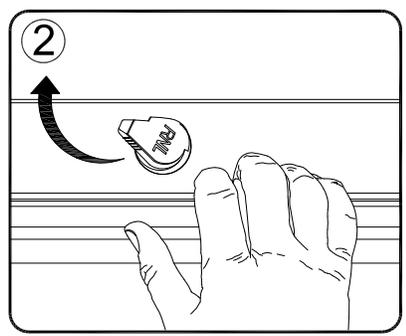
To open cover pull back on the handle, turn the lock to 10 o'clock and let the cover retract into the housing while holding onto the pull strap.
