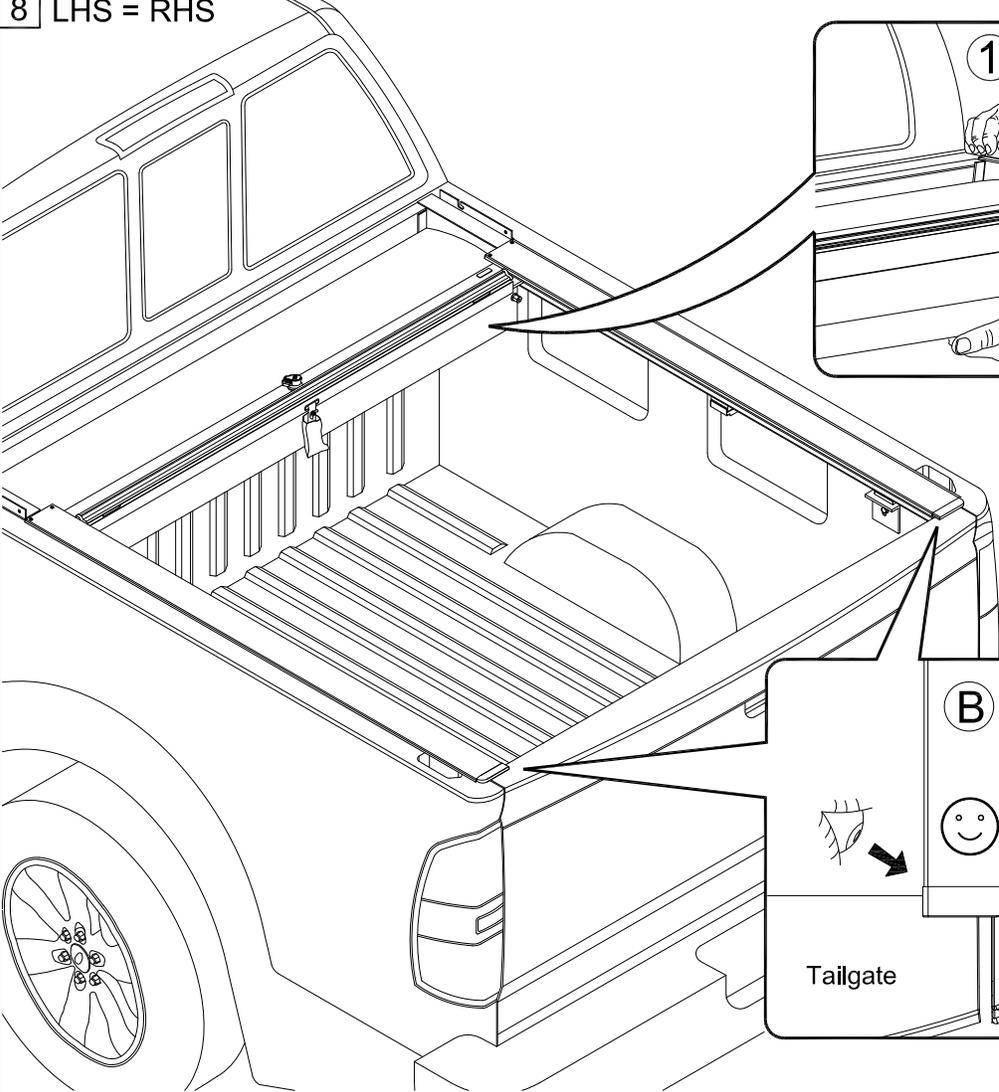
Close tailgate, shift the Housing back so the end of the Tracks are up against the tailgate.
