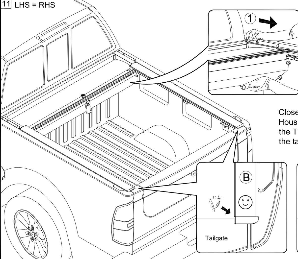
Close tailgate, shift the Housing back so the end of the Tracks are up against the tailgate.
