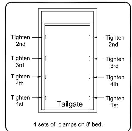
Tighten bed clamps to the track clamps. Note: When tight there may be a gap between the clamps, do not overtighten.
