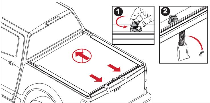
**11** Replace lid on housing (A) by lining up the pin with the slot and pushing down (1) and toward tailgate (2) on driver and passenger side. Then install the 1/4" lid screws (N) with a Phillips screwdriver (3) on driver and passenger side.
