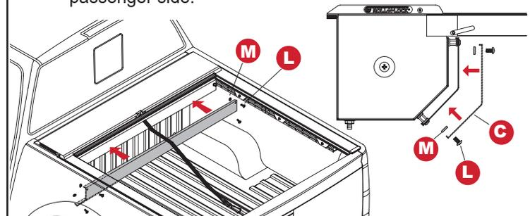
**14** Drill 1/2" hole (1) through bulkhead existing bed plug as shown. **DO NOT** drill through the truck bed cab. Insert one end of the drain tube (E) through the 1/2" drilled hole and feed toward the ground and insert the other end into the housing fitting on driver and passenger side. Make sure the drain tubes (E) are NOT aligned with or through the cab vents (1) on driver and passenger side. **Note:** Rust protection should be used on the holes you drilled.
