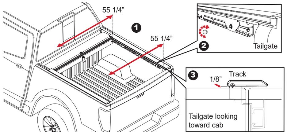
**10** Turn lock to 7 o'clock (1), remove plastic wing nut (2) and using both hands pull cover back to tailgate. (Discard plastic wing nut).
