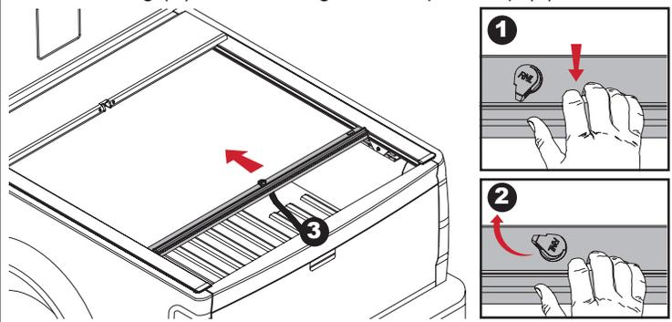
**13** **Note:** Remove the protective backing from the cargo shield (C) first. Attach cargo shield with the slots at the bottom of the housing (A) using two (2) black rubber washers (M) and two 1/4-20x3/8" screws (L) on driver and passenger side.
