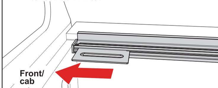
**NOTE:** Some drop-in bedliners may require trimming in the corners to fit the rail into the opening.
