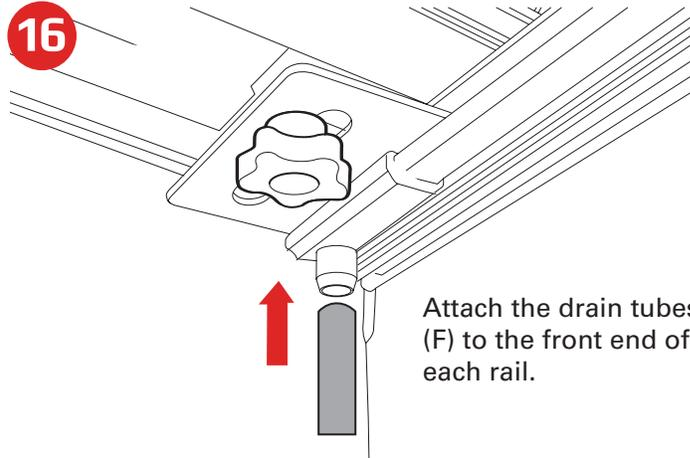
Attach the drain tubes (F) to the front end of each rail.
