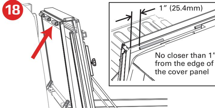
With the bed cover in the folded position, install the three D-shaped cab bumpers (E) along the top edge of the cover where it meets the truck cab.
