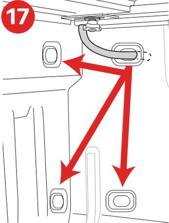
Route the other end of the drain tube (F) through the factory bed plug. Simply remove these plugs or drill a 7/8" hole through the plastic. Alternately, the plug can be trimmed using a utility knife making sure to cut a hole large enough to not crimp the drain tube. **NOTE:** If you have a drop-in bedliner, simply run the drain tubes behind or under the liner.
