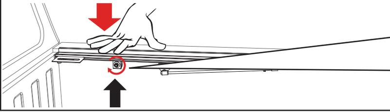
**NOTE:** When installing each clamp, make sure that the clamps are inserted as far up onto the rail as possible and that the clamp teeth fit squarely and fully engage the ribs of the cover rail.
