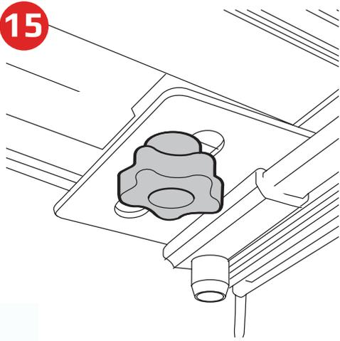
Once the cover is positioned correctly, fold the cover over toward the cab and tighten the knobs (L) until the lock washer (K) flattens out and locks the knob securely to the bracket.
