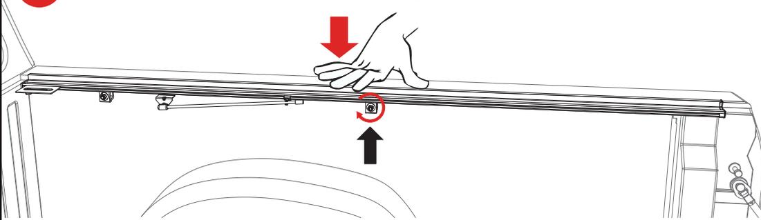
Always apply downward pressure to the cover rail when tightening the clamps to ensure that the rail sits flush and the seals are set.
