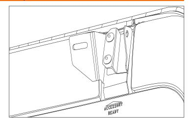
5. Install the L-Shaped bracket (#3-RH & #4-LH) over the light bar bracket using a 13mm socket. Repeat on the other side of the vehicle.
