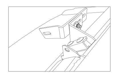
6. With assistance, install the Light Bar over the L Shaped bracket using the hardware provided with the Light Bar you have purchased. Repeat on the other side of the vehicle.
