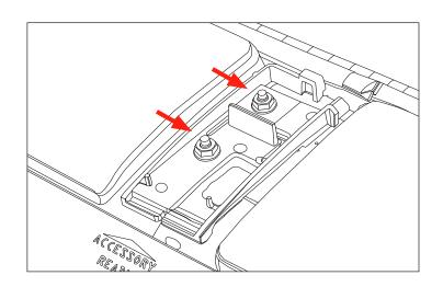
3. Install Light Bar Bracket (#1-RH & #2-LH) with provided M6 Barrel Nut (#7) using an allen wrench. Repeat on other side of the vehicle.
