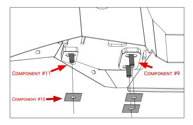
11. Using 8mm socket, remove OE bolts on inner cooler mounts. Install finishing plate, using OE hardware, to inner cooler mounts.
