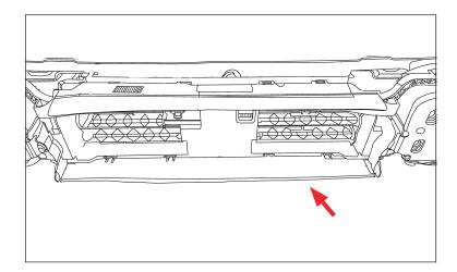
3. Remove the OE bumper nut plates from both sides by removing the plastic thumb screws.
