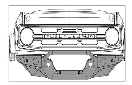
15. If required by state law, attach license plate bracket to bumper using M6 hardware. Reinstall OE wire harness if needed, use provided zip ties.
