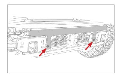
12. Using supplied M12 hardware, loosely attach bumper to frame horn.
