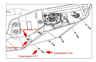
14. Center the bumper to the vehicle and tighten M12 hardware.
