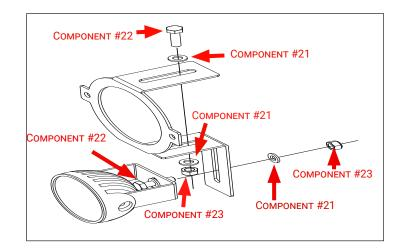
9. Loosely attach LED assembly to bumper. Align light in bumper recess and then tighten hardware.
