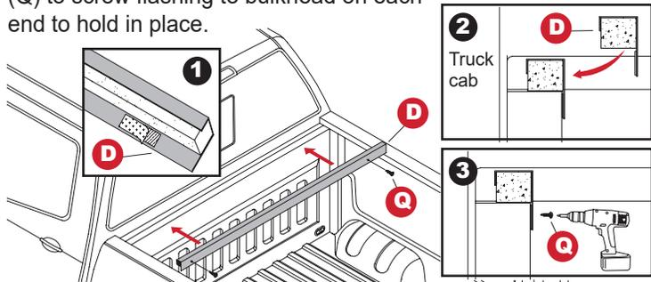
**3** Press butyl caulk strip (P) on top of bulkhead near side rail on both driver and passenger sides.
