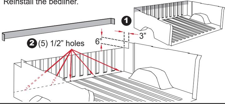
**1B** Drill 1/2" hole through plug (1) at bulkhead as shown with 1/2" drill bit with drill (2). DO NOT drill through the truck cab. Repeat on driver side. **Note:** Rust protection should be used on the holes you drilled.
