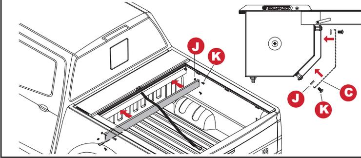
**17** Insert one end of the drain tube (D) through the 1/2" hole that was drilled through plugs (1) in step (1B) and insert the other end onto the housing fitting. Make sure the drain tubes (L) are NOT aligned with or through the inside of truck cab (2) on driver and passenger side.
