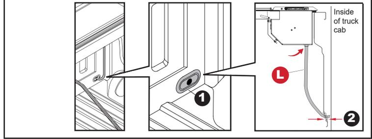
**18** Attach pull strap to the trucks rear driver or passenger side rear tie-down towards tailgate.
