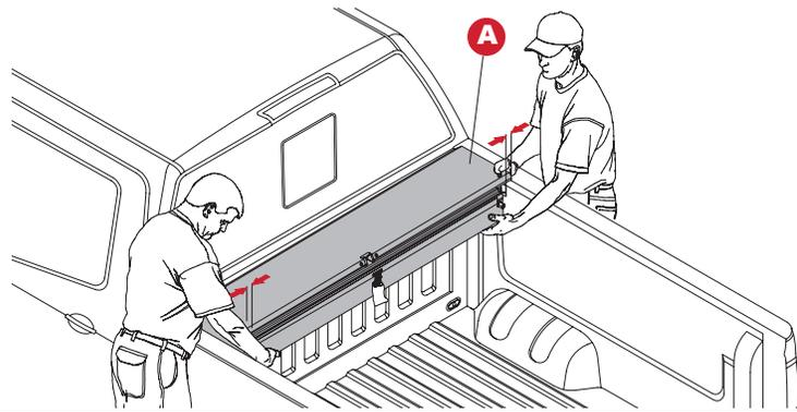
**5** Remove lid from housing (A) by pushing toward cab (1) and up (2) on driver and passenger side.
