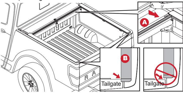
**10** Important to check track to track inside dimension, otherwise the cover will not latch properly on driver and passenger side.
