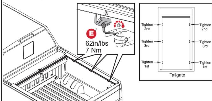
**12** If the tracks are not at a 90° degree angle you can use the 1/4-20x1" screw (N) and the 1/4-20 nut (O) to align the track to correct position.
