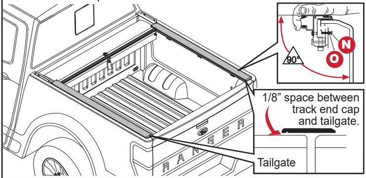
**13** Turn lock to 7 o'clock (1), remove plastic wing nut (2) and using both hands pull cover back to tailgate. **(Discard plastic wing nut).**
