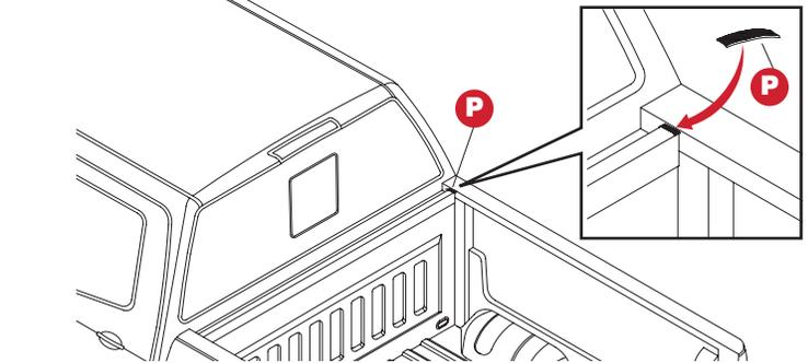
**4** Center the housing (A) between the bed rails, and up against the bulkhead on driver and passenger side.
