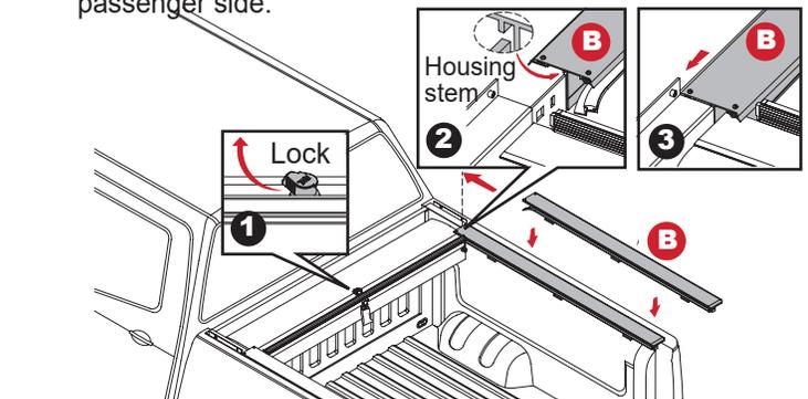
**7** Secure tracks (B) to housing stem (1) on driver and passenger side using cargo nut (G) and #10-24 screw (F) using a Phillips screwdriver (2).
