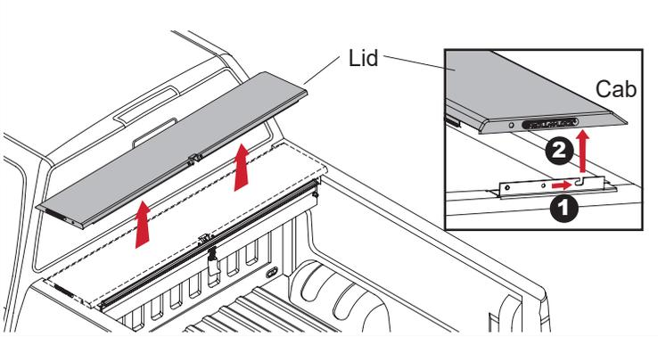
**6** (1) Turn lock to 10 o'clock. (Do not remove plastic wing nut). (2) Align tracks (B) onto housing stem. (3) Make sure the edge of the tracks butt up against housing on driver and passenger side.
