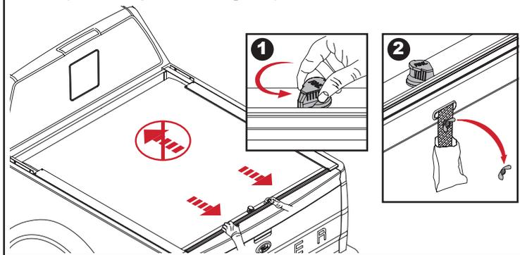
**14** Replace lid on housing (A) by lining up the pin with the slot and pushing down (1) and toward tailgate (2) on driver and passenger side. Then install the 1/4" lid screws (M) with a Phillips screwdriver (3) on driver and passenger side.
