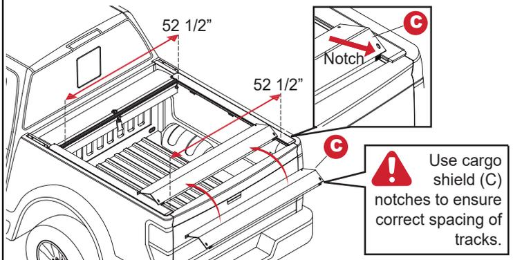
**11** Tighten bed clamps (E) to the pre-installed track clamps using a 1/4" Allen wrench on driver and passenger side. **Note:** When tight there may be a gap between the clamps, **do not over-tighten.**
