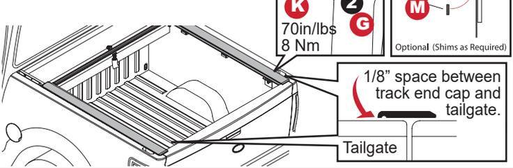
**12** Tighten bed clamps (L) to the pre-installed track clamps using a 1/4" Allen wrench on driver and passenger side. **Note:** When tight there may be a gap between the clamps, **do not over-tighten.**
