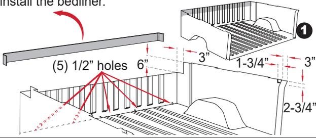
**1B** **FOR SUPER DUTY ONLY** - If there is No plastic bedliner proceed with step 1C. Like step (1A) using a tape measure follow the measurements in that step and mark on bedliner where to cut. Then use a jig saw to cut the liner parts out. In step (1A) the measurement is 3-3/4" (1) instead of 3". Drill (5) 1/2" holes where indicated. Repeat on driver side. Then mark on tailgate protector (2) where to cut and take it off tailgate to cut it. Discard cut parts. Replace tailgate protector.
