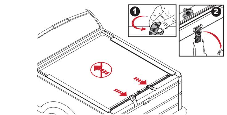
**14** Replace lid on housing (A) by lining up the pin with the slot and pushing down (1) and toward tailgate (2) on driver and passenger side. Then install the 1/4" lid screws (R) with a Phillips screwdriver (3) on driver and passenger side.
