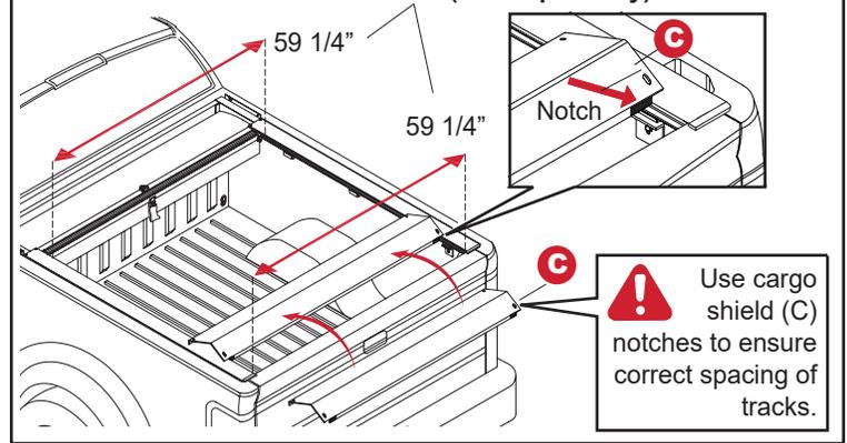
**11** Once tracks (B) are correctly spaced and adjusted to the correct height, tighten back clamp (E) with fastener (K) using 1/4" Allen wrench (1) and fastener (G) using a 7/16" wrench (2). You can use shim(s) (M) to align the track to 90° position on driver and passenger side.
