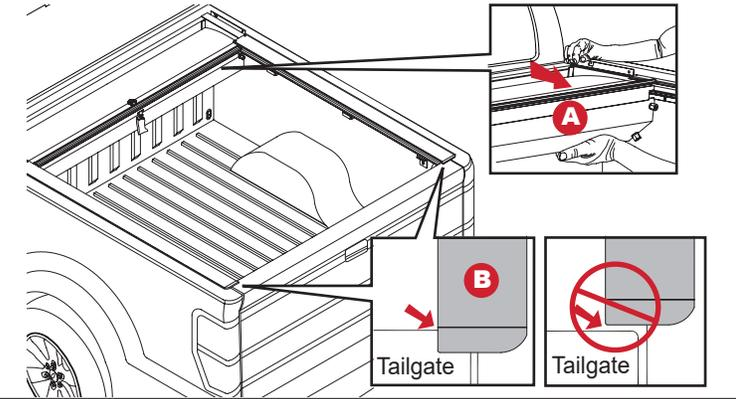
**10** Important to check track to track inside dimension, otherwise the cover will not latch properly on driver and passenger side.
