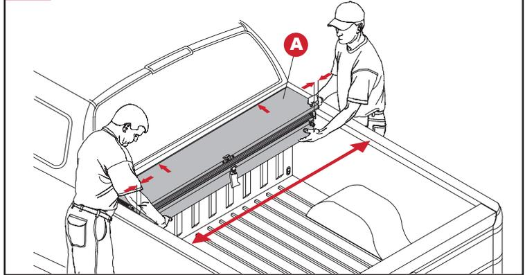
**3** Remove lid from housing (A) by pushing toward cab (1) and up (2) on driver and passenger side.
