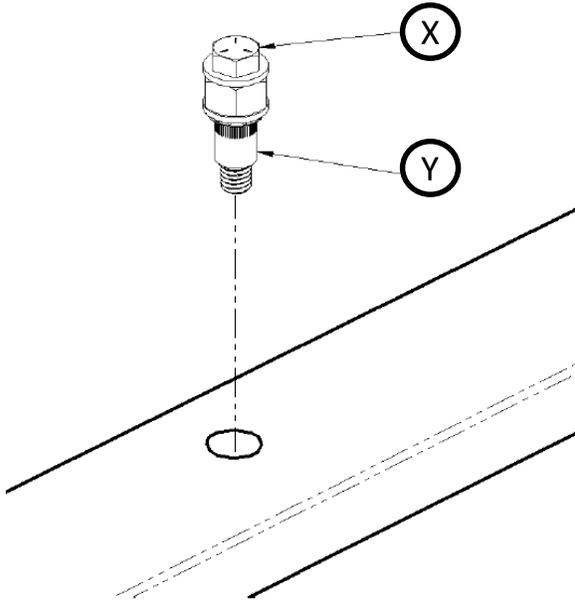
Drill 17/32" holes through top side of bed rails.
