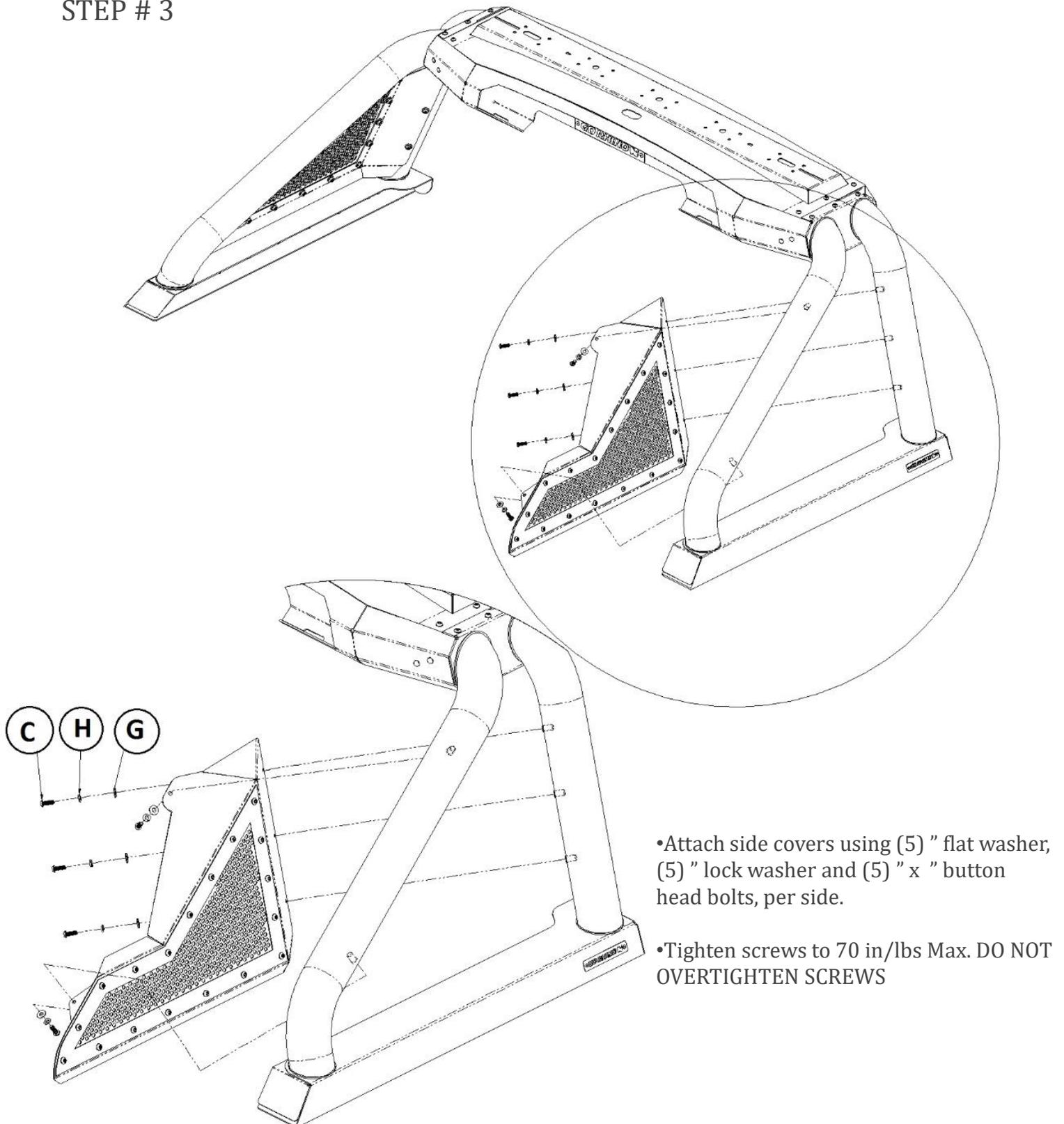
•Attach side covers using (5) " flat washer, (5) " lock washer and (5) " x " button head bolts, per side.
