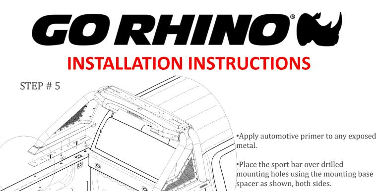
•Attach the sport bar using (3) 3/8" bolt plates and (3) $3/8" \ge 11/4"$  flat head bolts, per side.
