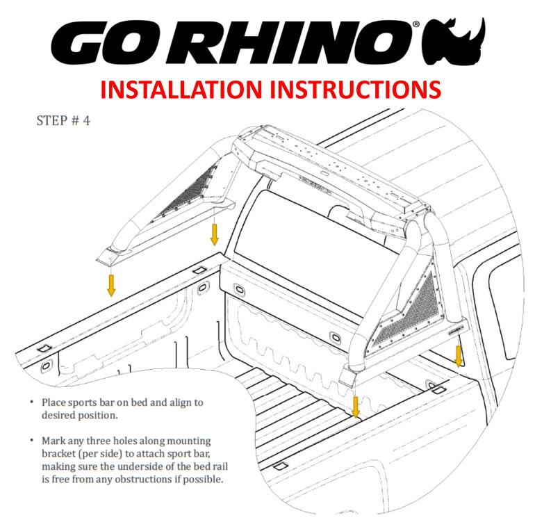
• Remove sport bar and drill 17/32" holes through bed rails.
