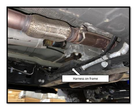
**Step 13**: Route the motor and LED wire harness from the controller to the Passenger side frame rail of the vehicle. When routing the harness keep clear from any moving parts and avoid direct contact with the exhaust system.
