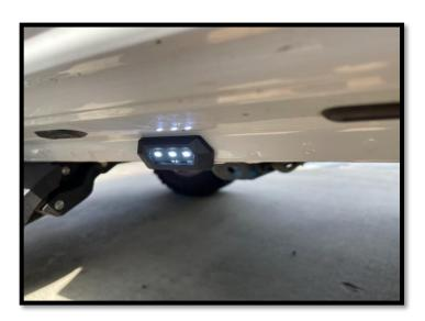
**Step 12**: Align the arrows on the small round connectors and plug the Passenger side front and Passenger side rear LED lights. Prepare the surface by cleaning with a 50/50 mix of isopropyl alcohol and water or equivalent. Once the surface is completely dry, peel the backing from the double-sided tape and stick the LEDs to the bottom side of the rocker panel. Position the LED lights at the center of the front and rear passenger side doors
