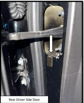
**Step 20:** With the rear driver side sensor attached, you can determine the correct position for the door magnet. peel the backing from the double-sided tape and stick the magnet on the door. Align the bottom of the magnet with the 4 1/2"
