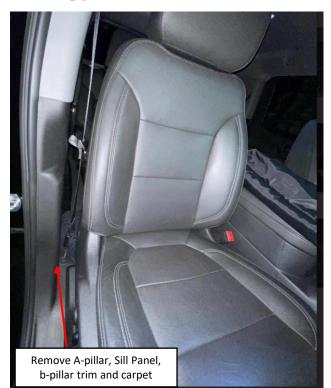
**Step 15:** Route the passenger side door trigger wire (brown) towards the passenger side bpillar. Route the driver side door trigger wire (white) and the black disable switch wires under the center console to the left side of the vehicle. The white wire needs to go to the driver side b-pillar, the black wires will go to the center console.
