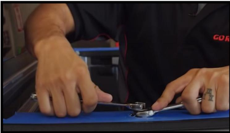
**STEP 15:** With the rivet nut positioned, use the provided rivet nut tool (item 25) to compress the rivet nut. Use a  $\frac{3}{4}$ " wrench to hold the spacer on the rivet nut tool and a  $\frac{9}{16}$ " wrench to turn the head of the rivet nut tool. This will compress the rivet nut. Once tight, unscrew the bolt and repeat the steps for the remaining rivet nuts. **OPTIONAL:** You can use an impact gun on the head of the rivet nut tool or rivet nut gun to compress the rivet nut.
