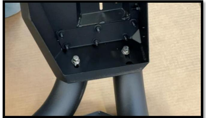
**STEP 6:** With assistance, install box assembly onto front and rear tubes as shown. Position the rear upper vinyl washer (item 14) and front upper vinyl washer (item 13) in between the tubes and base plate. Fasten down using 3/8" hex bolts (2), 3/8" flat washer (2) and 3/8" lock washer (2). Leave finger tight for later adjustment. Repeat steps for passenger side.
