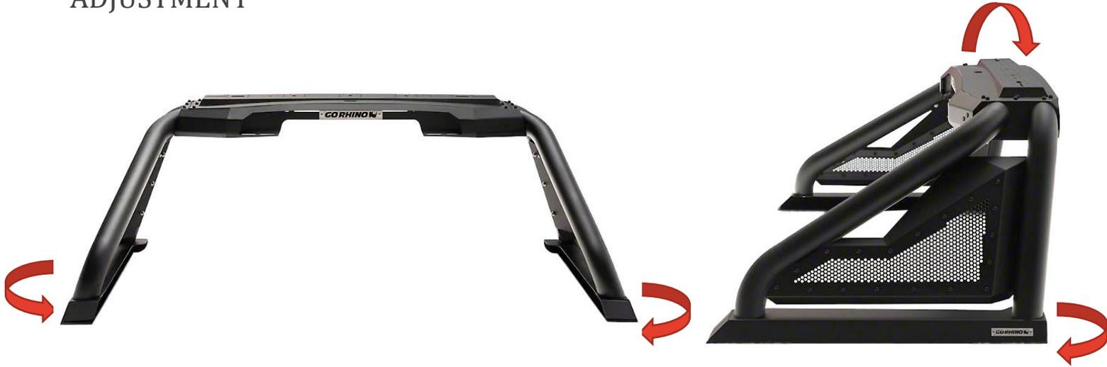
**STEP 7:** In some cases, the Sport Bar 2.0 may appear to sag or be too wide for some applications. This is normal as it comes with multiple points of adjustments which are finalized during the install. For this reason, it is recommended to leave all the hardware hand tight during the assembly process.
