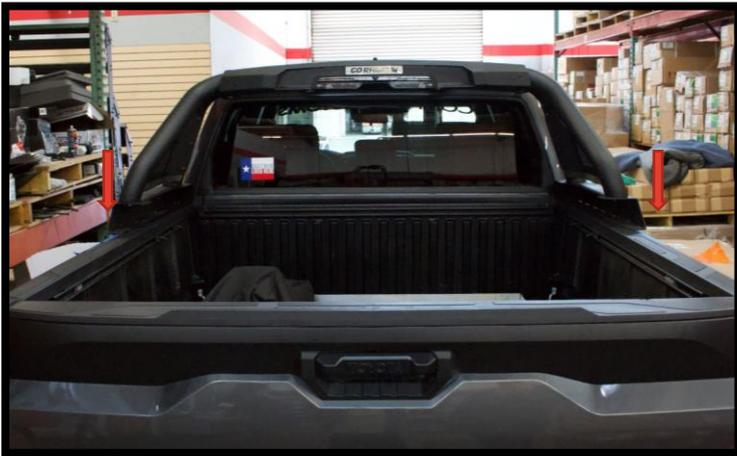
**STEP 17:** Place the sport bar over drilled mounting holes using the mounting base spacer as shown, both sides. If hole was drilled through top and bottom, attach the sport bar using (3)  $\frac{3}{8}$ " flat washers, (3)  $\frac{3}{8}$ " lock washers and (3)  $\frac{3}{8}$ " x  $1\frac{1}{4}$ " flat head bolts, per side. If rivet nuts were installed, attach the sport bar using (3)  $\frac{3}{8}$ " x  $1\frac{1}{4}$ " flat head bolts, per side. Make any final adjustments that may be needed.
