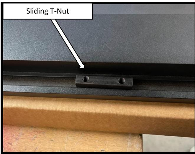
**Step 8:** Install the Passenger side running board. With assistance, begin by positioning the board on the front and rear motor assembly bases. Align the sliding T-Nut on the running board with the slots on the front and rear motor base. Once the T-Nuts are aligned, rotate the running board so that the T-Nuts set in the slots on the base of the arms. Repeat Steps 3-6 to install the motor linkage assemblies and running board on the Passenger side.
