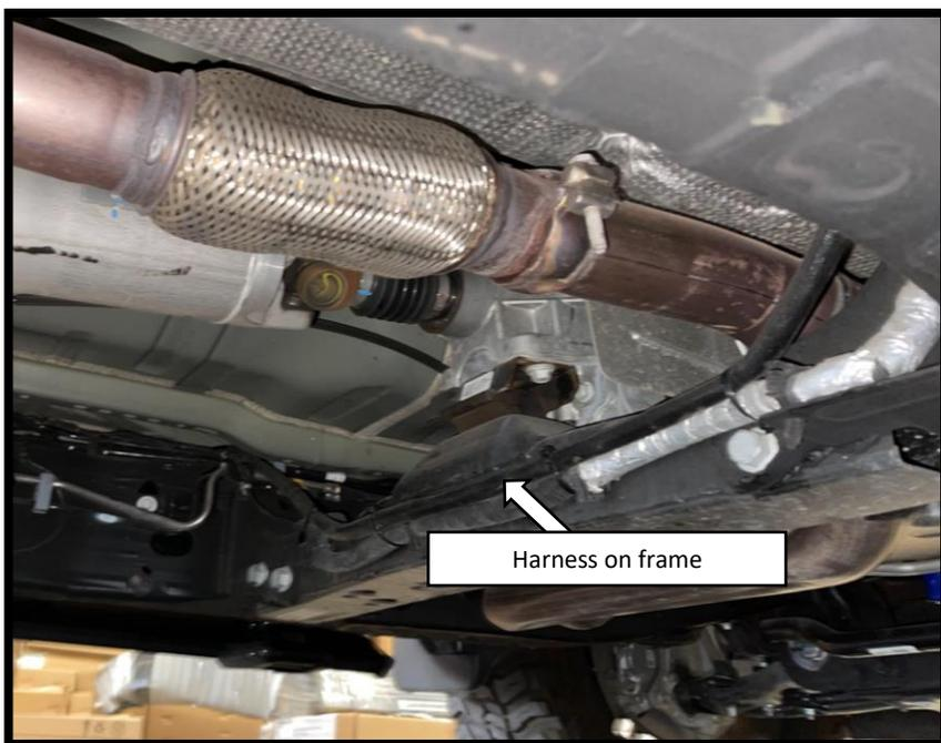
**Step 13:** Route the motor and LED wire harness from the controller to the Passenger side frame rail of the vehicle. When routing the harness keep clear from any moving parts and avoid direct contact with the exhaust system.
