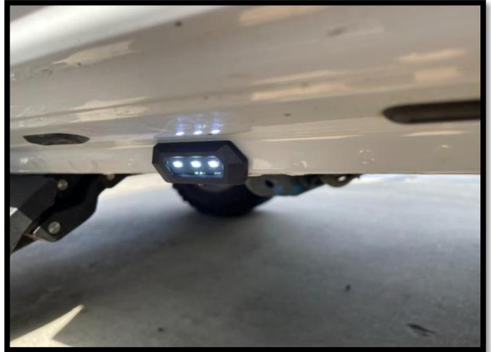
**Step 12:** Align the arrows on the small round connectors and plug the Passenger side front and Passenger side rear LED lights. Prepare the surface by cleaning with a 50/50 mix of isopropyl alcohol and water or equivalent. Once the surface is completely dry, peel the backing from the double-sided tape and stick the LEDs to the bottom side of the rocker panel. Position the LED lights at the center of the front and rear passenger side doors
