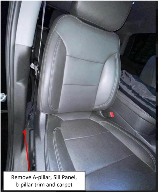
**Step 15:** Route the passenger side door trigger wire (brown) towards the passenger side b-pillar. Route the driver side door trigger wire (white) and the black disable switch wires under the center console to the left side of the vehicle. The white wire needs to go to the driver side b-pillar, the black wires will go to the center console.
