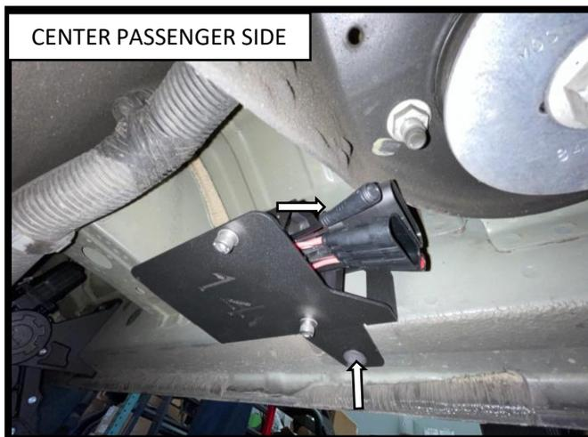
**Step 7:** Locate the threaded stud cluster near the center of the cab on the passenger side of the truck. Install the controller bracket using (2) M8X25mm Hex Bolts to fasten the motor to the truck.
