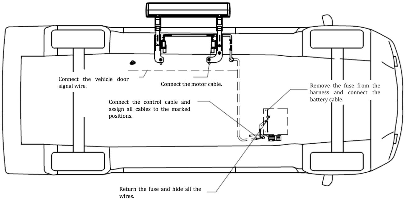
**Step 9:** Remove the fuse from the harness and connect the battery cable..
