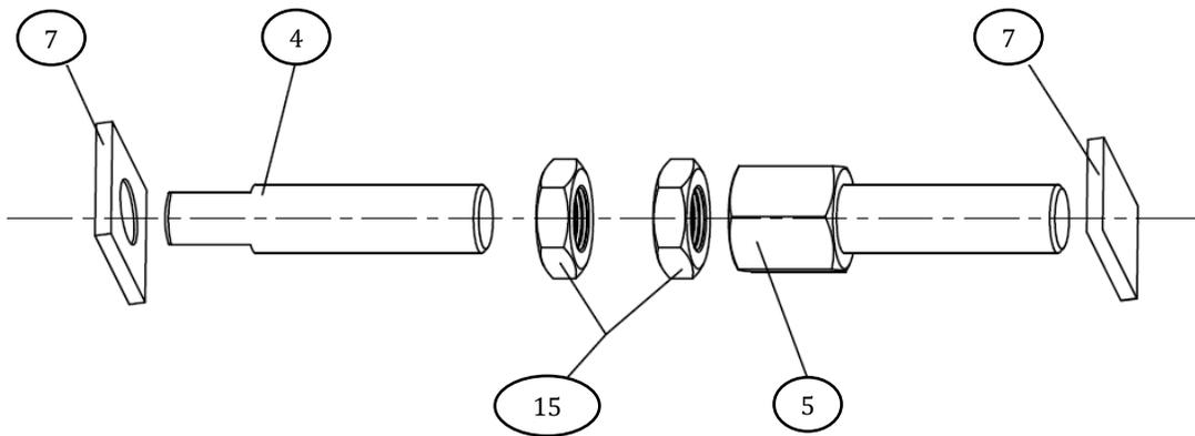
**Paso 5:** Place the stud and bolt assembly into the main bracket holes, adjust as necessary with the remaining M16 nuts in the center of the assembly
