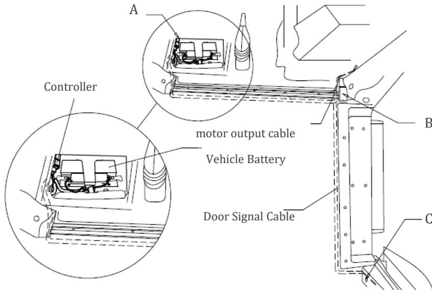
**Step 10:** Remove the carpet cover, and then arrange the control input cable as shown with the dotted line, pass the motor output cable through position B in the figure, and then pass the motor output cable to through the vehicle floor until you reach the bottom of the vehicle.
