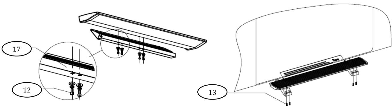
**Step 8:** Separate the T-nuts that are inside the bracket and place the bracket on the brackets as shown in illustration 8. Secure with M6 x 25mm screws, M6 flat washer and pressure washer.
