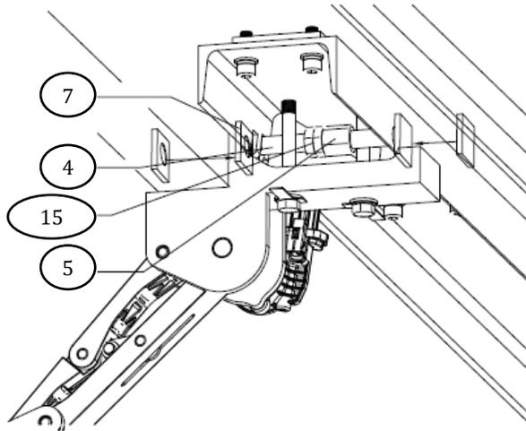
**Step 7:** Position the square spacer as shown in Figure 7, and then turn the adjusting nut to press the square spacer against the slot in the chassis. Place the Board Fender on the T-Nuts inside the foot peg and secure with M6 x 20mm bolts, M6 flat washer and M6 lock washer, as shown in illustration 8. NOTE: Make sure the Fender is centered
