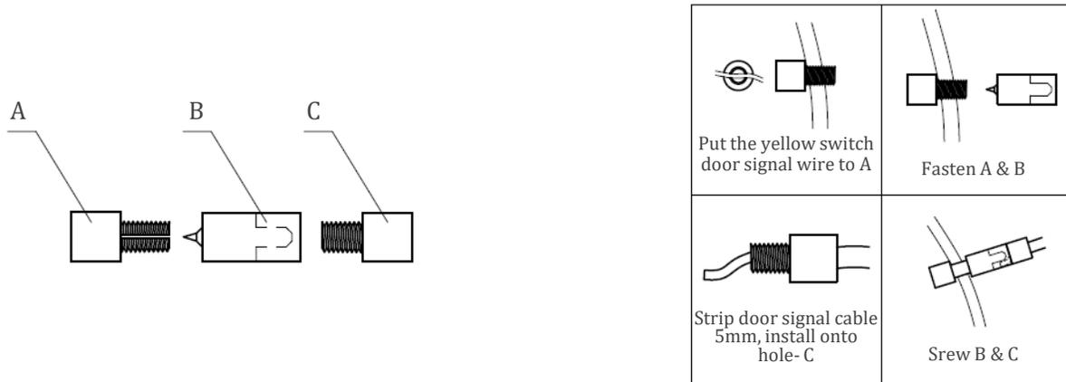
**Step 13:** Find the vehicle door signal wire (yellow color) and make the front part of the wire connector stick on the yellow wire. Make the middle of the cable connector puncture the yellow cable and tighten it. And then strip 5mm of the vehicle door signal wire (white color) and run the vehicle door signal from the end of the wire connector to the middle of the wire connector and tighten it.
