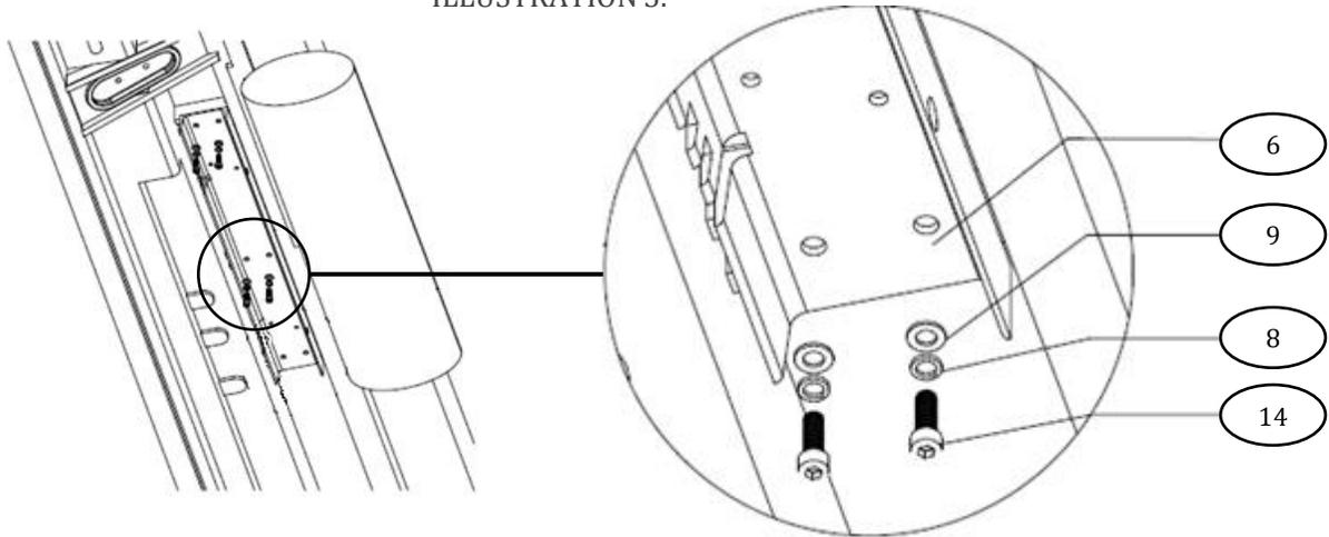
**STEP 3:** Place the BOARD brackets on the main bracket as shown in illustration 4. Secure with: 2 hex head screws. M8 x 100mm, 2 flat and pressure washers M8
