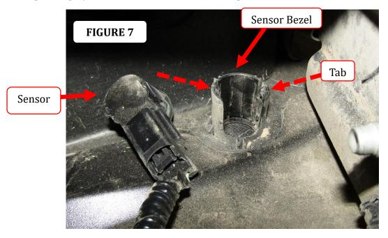
**Step-8** Remove the sensor bezels from the OEM bumper by depressing the (2) tabs around the base and pushing the bezel out through the front of the bumper, (FIGURE6). Note: The bezels have to be positioned in the bumper replacement in the same location (inner and outer), (driver and passenger) as removed from the OEM bumper.
