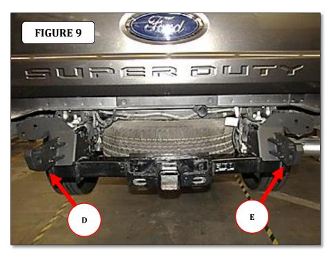
**Step-9** With assistance attach the bumper replacement bracket to each frame bracket and the OEM bumper bracket using (2) ½" x 2" hex bolts, (4) ½" flat washers, (2) ½" lock washers and (2) ½" Hex nuts, (FIGURE 10).
