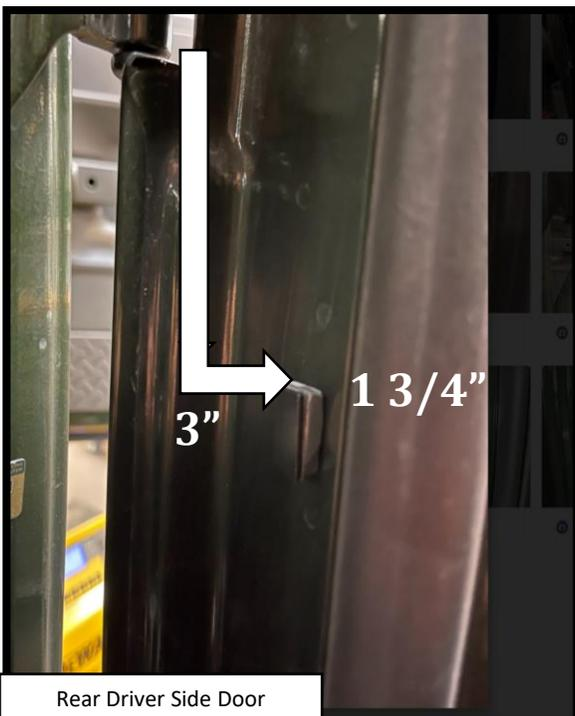
**Step 24** Install rear larger magnets a vertically oriented 3" from the bottom of the door hinge and 1 3/4" out to the inside corner of the door skin. Prepare the surface by cleaning with a 50/50 mix of isopropyl alcohol and water or equivalent. Once the surface is completely dry, peel the backing from the double-sided tape and stick the magnet to the door as shown. Verify that the magnet should be in line with the door sensor.
