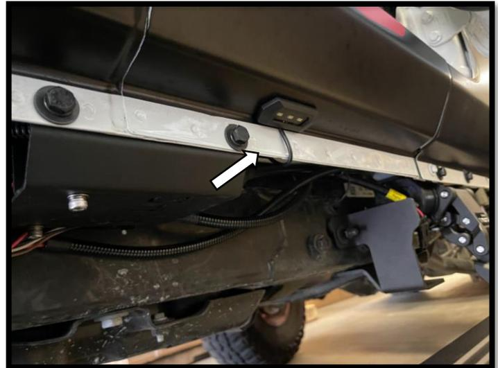
**Step 16:** Align the arrows on the small round connectors and plug the Passenger side front and Passenger side rear LED lights. Prepare the surface by cleaning with a 50/50 mix of isopropyl alcohol and water or equivalent. Once the surface is completely dry, peel the backing from the double-sided tape and stick the LEDs to the bottom side of the rocker panel. Position the LED lights at the center of the front and rear passenger side doors
