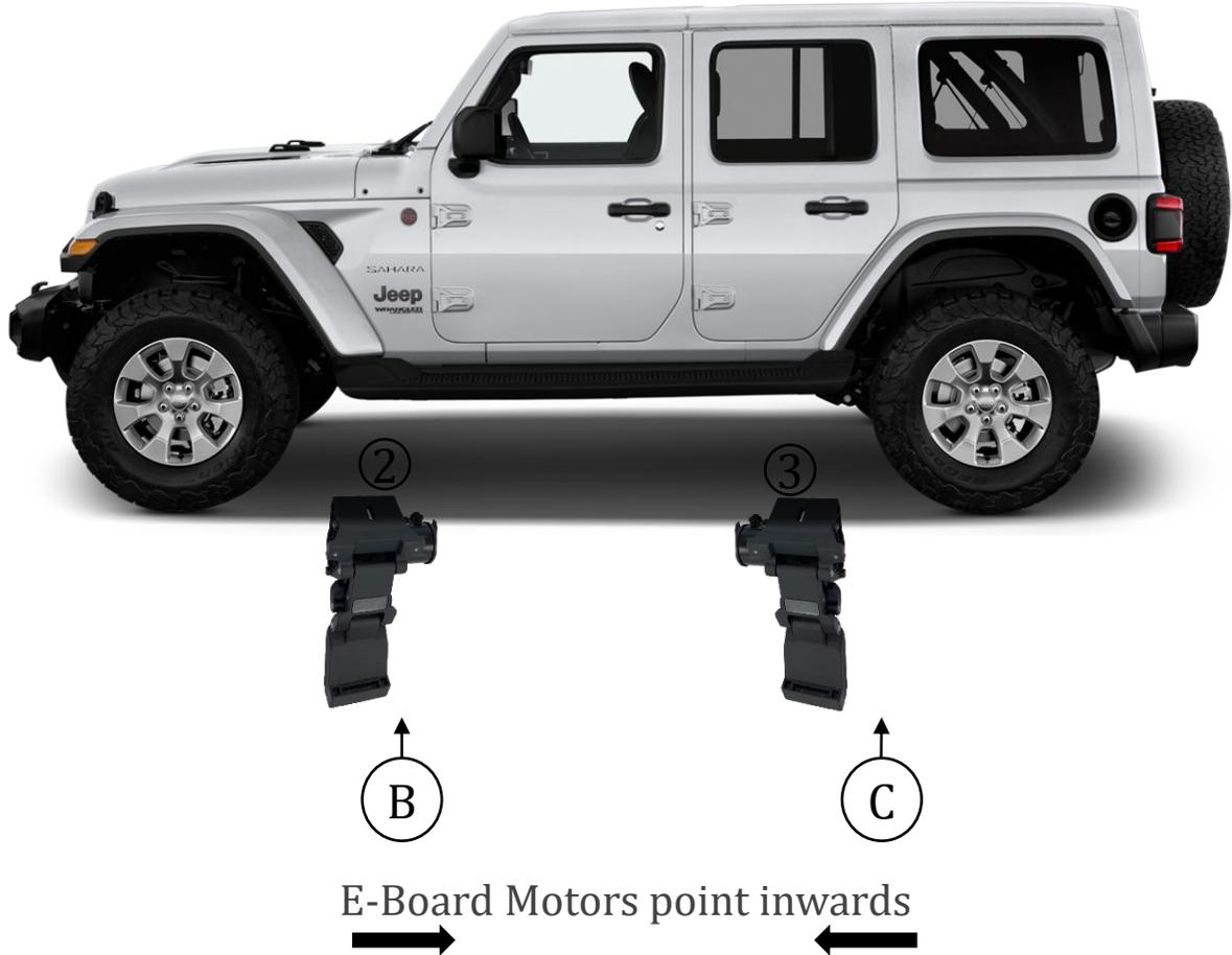
**Step 14:** Repeat Steps 1-11 to install the motor linkage assemblies and running board on the driver side.
