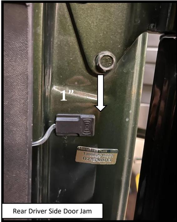
**Step 23: REAR DOOR** Install rear sensor about 1" from the lowest point of the door hinge. Prepare the surface by cleaning with a 50/50 mix of isopropyl alcohol and water or equivalent. Lift the bulb door seal to route the sensor wire underneath it. Once the surface is completely dry, peel the backing from the double-sided tape and stick the rear door sensor to the door jamb as shown.
