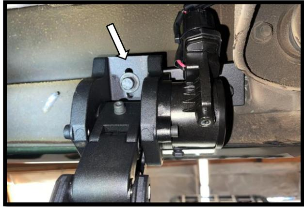
**Step 6:** . Install rear passenger side bracket onto weld seam using (2) M8x20MM Hex Bolts, M8 Lock Washer, M8 Flat Washer. On the underside of the bracket, secure it to the motor to the mounting plate using (1) M8x35MM Hex Bolts, M8 Lock Washer, M8 Flat Washer.
