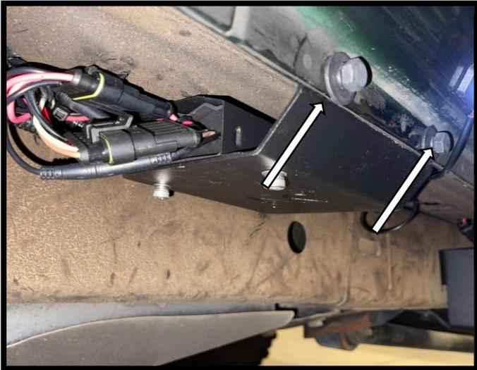
**Step 11:** Find the middle two holes on the pinch seam below the passenger side front door. Using two M8 hex head bolts, M8 flat washers and M8 lock washers, install the controller mounting bracket. Using a torque wrench, tighten to 18 ft-lb.
