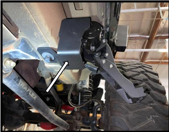
**Step 10:** Install the passenger side front motor protective bracket. Secure the protective bracket using an M12 hex bolt, flat washer, and lock washer. Torque to 25 ft-lbs.
