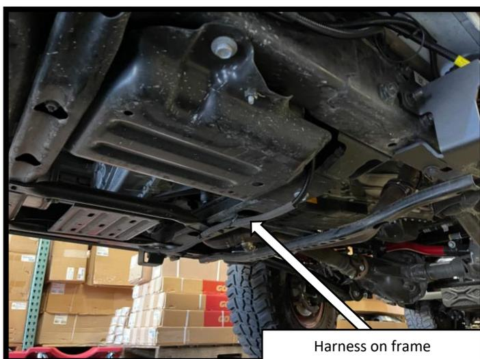
**Step 17:** Route the motor and LED wire harness from the controller to the Passenger side frame rail of the vehicle. When routing the harness keep clear from any moving parts and avoid direct contact with the exhaust system.
