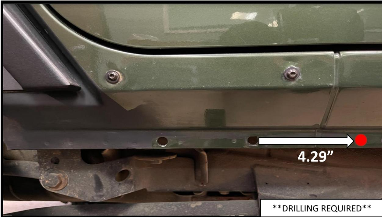
**Step 5:** . Using a measuring tape, measure 4.29" from the forward mounting hole. Use a center punch to mark the hole location and drill the 21/64" hole. Use touch up paint to cover up any raw metal on the pinch seam. You can check to see if you placed the hole in the correct location by mocking the bracket up against the weld seam
