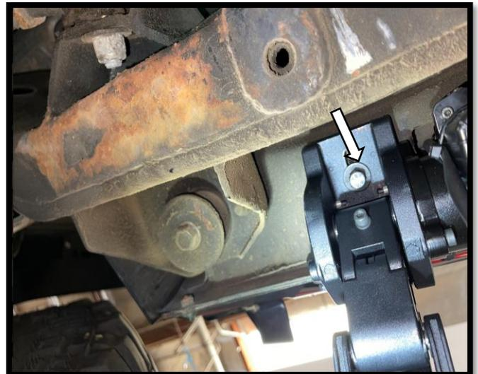
**Step 8:** . Install front passenger side bracket onto weld seam using (2) M8x20MM Hex Bolts, M8 Lock Washer, M8 Flat Washer. On the underside of the bracket, secure it to the motor to the mounting plate using (1) M8x35MM Hex Bolts, M8 Lock Washer, M8 Flat Washer.
