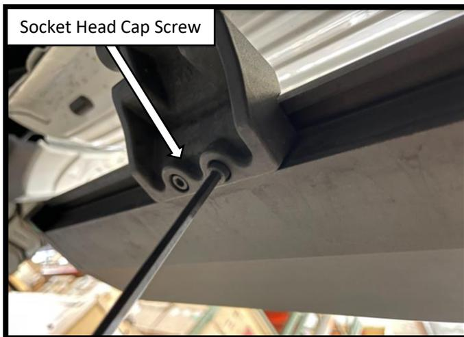
**Step 8:** Determine where you want to position the board and secure the running board to the arms using the (2 per bracket) M6x25 socket head cap screws. Using a torque wrench, tighten to 9 ft-lbs. Step # With the running board is installed, fasten the hardware on the Driver side front and rear motor assemblies. Using a torque wrench, tighten the mounting hardware to 18 ft-lbs.
