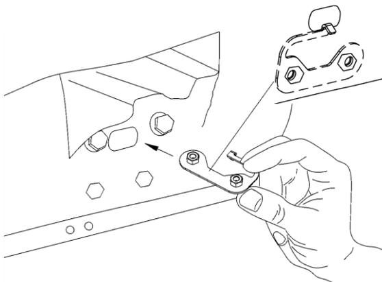
**Step 3 :** Install the Front Driver side motor using (1) Nut Plate , (2) M8 Hex Bolts. Holes that do not have factory threaded inserts will require the threaded nut bracket that is included in this kit. The hardware should be hand tightened only until snug. This will allow the motor assembly to move and align easier when installing the running board.
