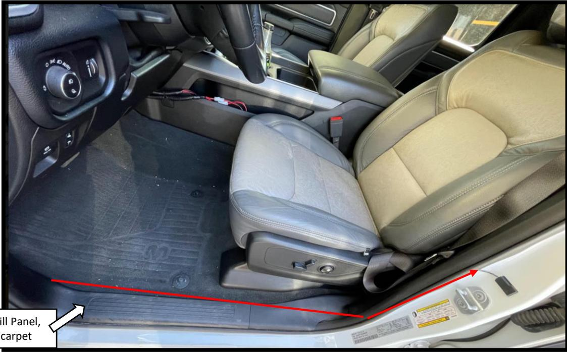
**Step 15:** Route the Driver side door trigger wire (brown) towards the Driver side b-pillar. Route the Passenger side door trigger wire (white) under the center console and over to the Passenger side b-pillar. Route the black disable switch wires to the center console.
