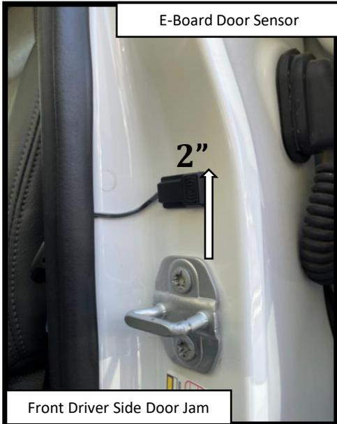
**Step 17:** FRONT DOOR: With the weatherstrip peeled back, route the sensor wire underneath it. Clean the surface by cleaning with a 50/50 mix of isopropyl alcohol and water or equivalent. Once the surface is completely dry, peel the backing from the double-sided tape and stick the sensor on the door jamb. Align the top of the sensor with the 2"
