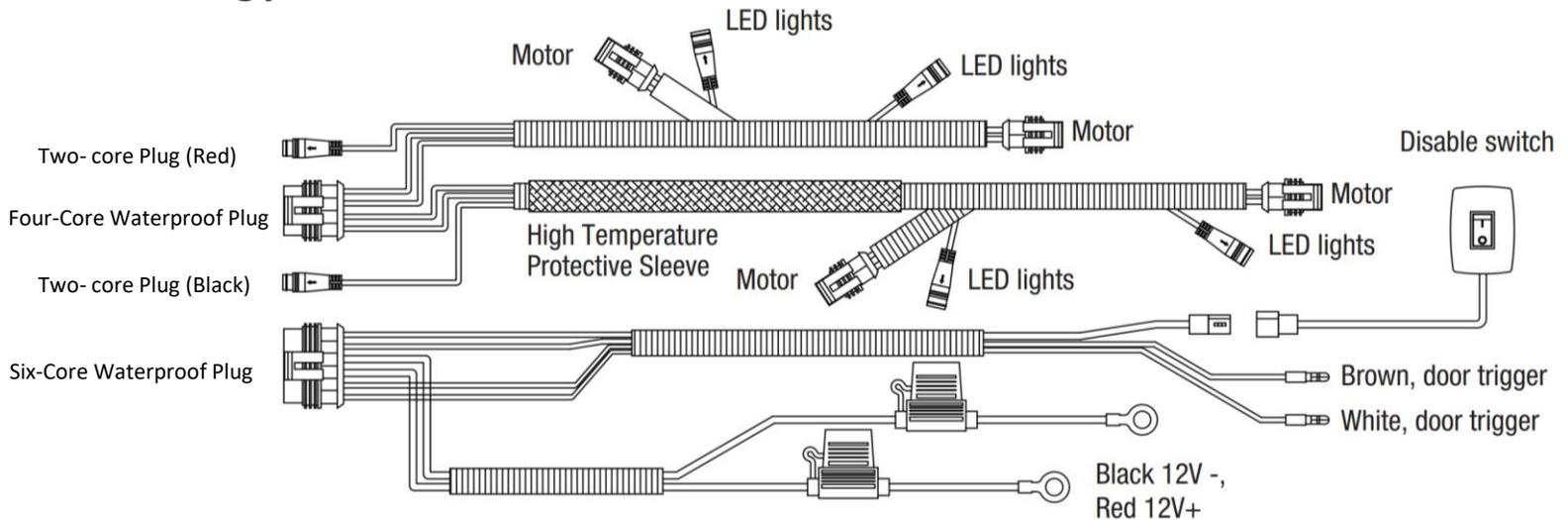
**Step 10:** Route the electrical harness from the controller along the frame rail of the truck. Connect the male plug connector on the wire harness into the female socket on the motors. The harness is labeled to show where to plug each male connector to the female connector. For example, Front Left is for the front Driver side motor and Rear Left for the rear Driver side motor. Use supplied zip-ties to secure harness to the frame rail.
