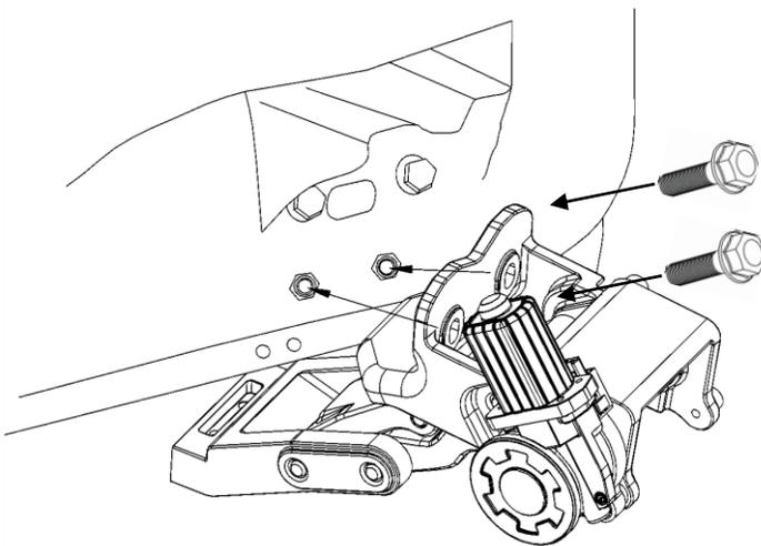
**Step 4:** Install the rear Driver side motor using (1) Nut Plate , (2) M8 Hex Bolts. Holes that do not have factory threaded inserts will require the threaded nut bracket that is included in this kit. The hardware should be hand tightened only until snug. This will allow the motor assembly to move and align easier when installing the running board.
