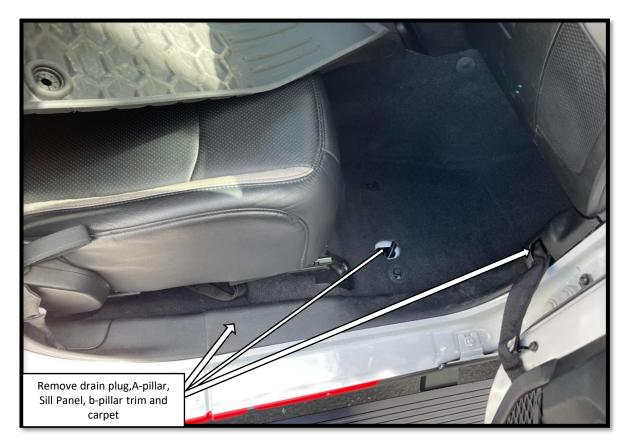
**Step 18:** Go under the vehicle and feed the door trigger signal wires (white and brown) and the disable switch wires (two black wires) into the cab. Feed the wires thru the hole in the rubber drain plug. Pop the drain plug back into the slot. Seal around the wires using RTV silicone adhesive to prevent water intrusion.
