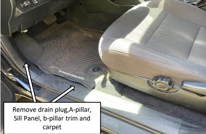
**Step 13:** On the DRIVER side, remove the front kick panel, front door sill trim panel and b-pillar trim panel. Go under the passenger seat and locate the split in the carpet. Pull the rear half of the carpet back to expose the oval rubber drain plug. Pull the drain plug and drill a 7/16" hole.
