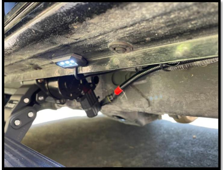
**Step 11:** Align the arrows on the small round connectors and plug the Passenger side front and Passenger side rear LED lights. Prepare the surface by cleaning with a 50/50 mix of isopropyl alcohol and water or equivalent. Once the surface is completely dry, peel the backing from the double-sided tape and stick the LEDs to the bottom side of the rocker panel. Position the LED lights at the center of the front and rear passenger side doors
