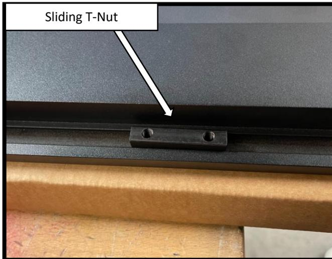
**Step 6:** Install the DRIVER side running board. With assistance, begin by positioning the board on the front and rear motor assembly bases. Align the sliding T-Nut on the running board with the slots on the front and rear motor base. Once the T-Nuts are aligned, rotate the running board so that the T-Nuts set in the slots on the base of the arms. Repeat 1-14 to install the motor linkage assemblies and running board on the PASSENGER side side.
