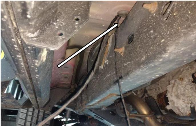
**Step 14:** Go under the vehicle and feed the door trigger signal wires (white and brown) and the disable switch wires (two black wires) into the cab. Feed the wires thru the hole in the rubber drain plug. Pop the drain plug back into the slot. Seal around the wires using RTV silicone adhesive to prevent water intrusion. These cables will run underneath the driver side seat.
