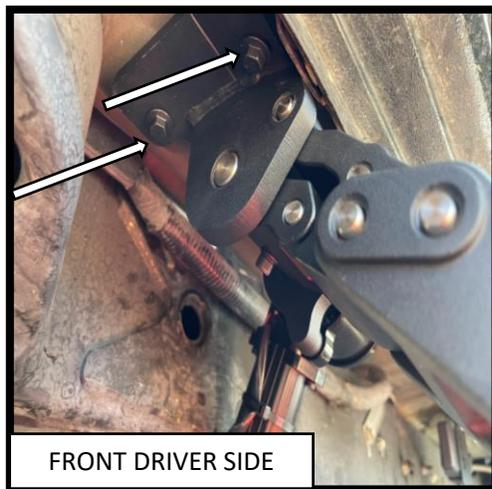
**Step 4:** Install the FRONT DRIVER side motor using (2) M8X30mm Flange Bolts, to fasten the motor to the vehicle. The hardware should be hand tightened only until snug. This will allow the motor assembly to move and align easier when installing the running board.
