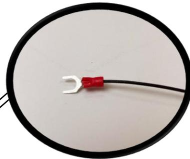
**Step 16:** The door trigger sensor harness will need a ground connection to the vehicle. Locate the seat belt assembly at the passenger side b-pillar and install the ground wire under the top bolt of the seat belt assembly.
