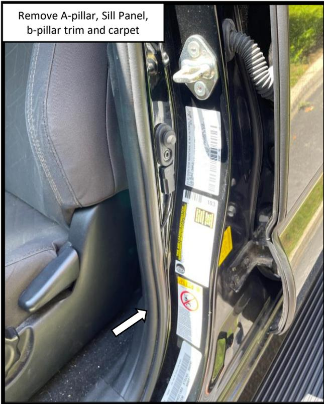
**Step 15:** Route the DRIVER side door trigger wire (brown) towards the DRIVER side b-pillar. Route the PASSENGER side door trigger wire (white) and the black disable switch wires under the center console to the left side of the vehicle. The white wire needs to go to the driver side b-pillar, the black wires will go to the center console.
