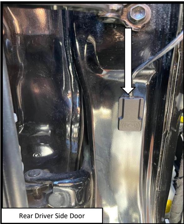
**Step 20:** With the rear driver side sensor attached, using the door stopper as a reference point. Make a mark 3.5" below the center line of the latch. Prepare the surface by cleaning with a 50/50 mix of isopropyl alcohol and water or equivalent. Once the surface is completely dry, peel the backing from the double-sided tape and stick the magnet to the door. Align the top of the magnet with the 3.5" mark as shown.
