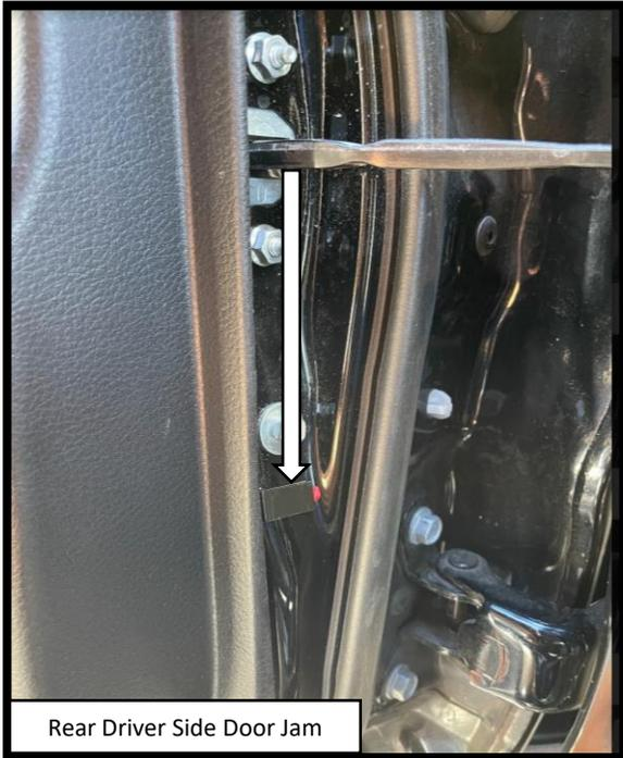
**Step 19: REAR DOOR** Apply a vertically oriented strip of masking tape on the rear Driver side door using the door stopper as a reference point. Make a mark 3.5" below the center line of the latch. Prepare the surface by cleaning with a 50/50 mix of isopropyl alcohol and water or equivalent. Once the surface is completely dry, peel the backing from the double-sided tape and stick the magnet to the door. Align the top of the magnet with the 3.5" mark as shown.
