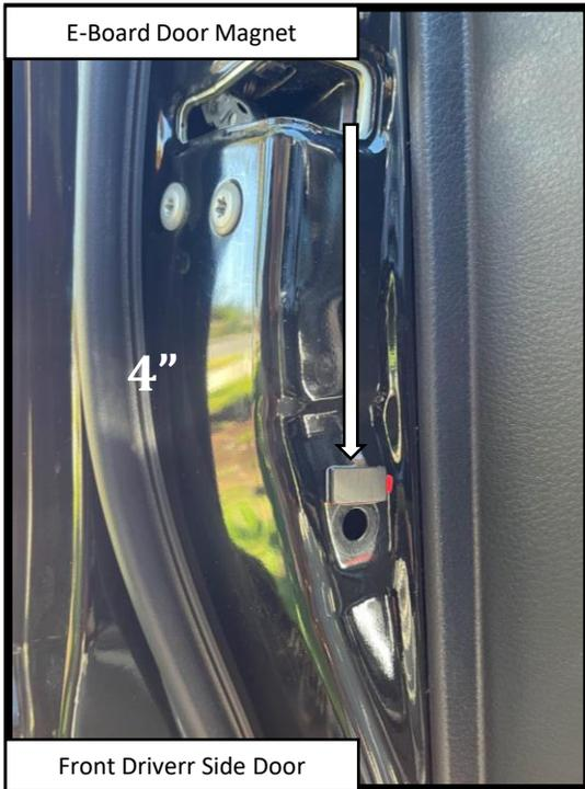
**Step 17: FRONT DOOR** Apply a vertically oriented strip of masking tape on the front Driver side door using the deepest part of the latch as a reference point. Make a mark 3.5" below the center line of the latch. Prepare the surface by cleaning with a 50/50 mix of isopropyl alcohol and water or equivalent. Once the surface is completely dry, peel the backing from the double-sided tape and stick the magnet to the door. Align the top of the magnet with the 4" mark as shown.
