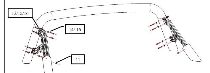
Step 2: Install the front and rear plastic cover with ST4.2\_30.
