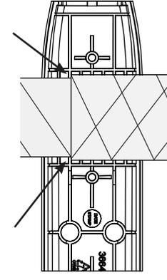
**7** **NOTE:** The inside of the upright is stepped to fit correctly around the small and large diameter tubes.
