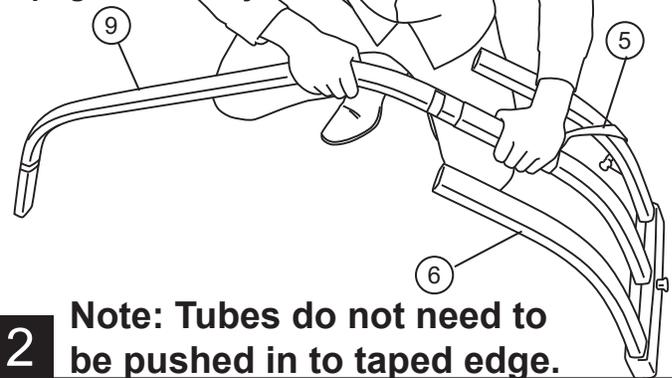
**Note: Tubes do not need to be pushed in to taped edge.**
