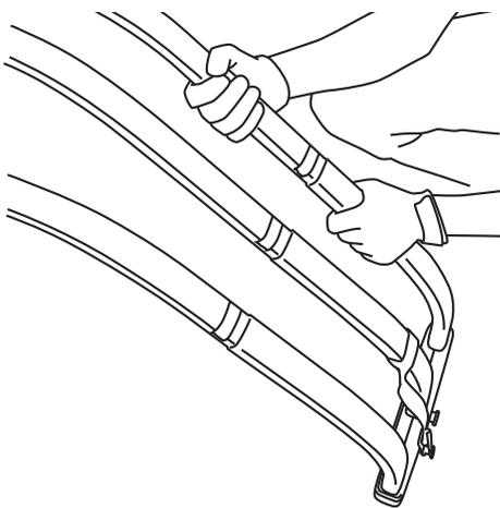
**Note: Install Strap Buckle Assembly to center tube of Pivot Upright Assembly.**
