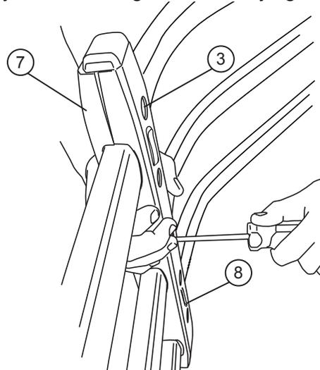
**7** NOTE: The inside of the upright is stepped to fit correctly around the small and large diameter tubes.
