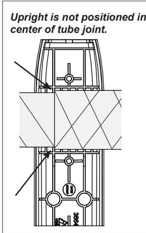
Tighten PT-Screws using a T-25 torx driver, starting in the middle of each upright, then the outer screws and lastly the remaining two to evenly tighten.
