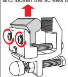
Re-tighten screws and fully engage the lock washers.
