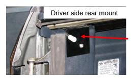
Start rear mounting screws. Slide a flat washer onto the (2) M6 x 40mm (metric) rear mount bolts, insert bolts through holes in rear rail brackets, then insert nylon spacer and start threading into factory holes at rear. Use 4mm Allen wrench.
