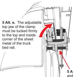
**5 Atl. f.** If the jaw does not contact firmly into the corner of the bed flange, remove the clamp and loosen the screws to adjust the jaw.
