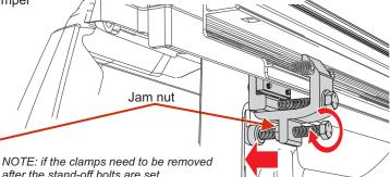
after the stand-off bolts are set, the jam nut and bolt will have to be loosened.
