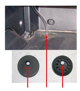
You can pass the tubes through the 2 factory plastic bed bolt covers. Remove the covers and drill a loose 1/2" hole or a 9/16' hole for the tubes. Offset the holes as shown.
