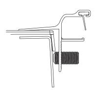
If the rails measured to be too close together, turn the screws counter clockwise.
