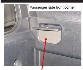
Remove the adhesive backing paper from the foam fillers for the tie-downs. Push into place over the tie-down bolts. Repeat on driver's side.
