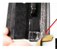
Remove the adhesive backing paper from under the front of both rails.
