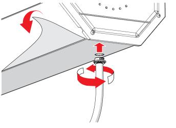
**9c.** Generally the drain tubes will be routed out through a hole drilled in the factory bed plug. Otherwise a suitable existing hole must be utilized. Or a new hole can be drilled, taking great caution to be aware of lines and anything behind where the hole is drilled.
