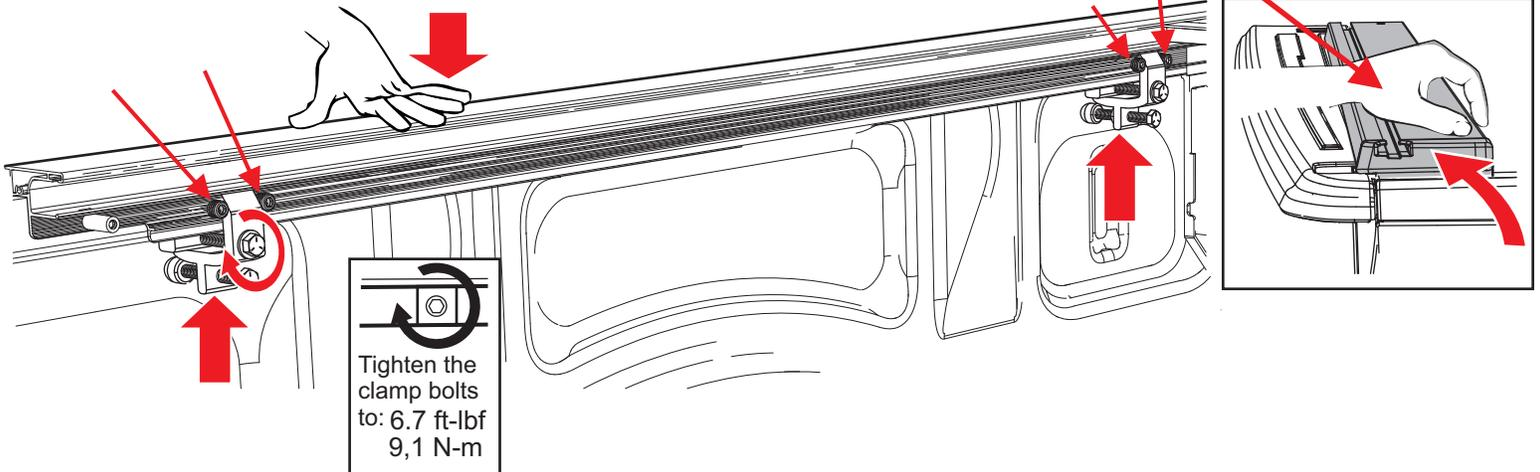
Tighten the clamp bolts to: 6.7 ft-lbf
