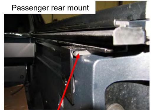
The rubber spacer provided can be added under the passenger rear mount bracket for proper clearance over the tailgate protector.
