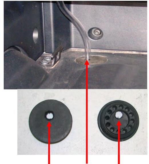
You can pass the tubes through the 2 factory plastic bed bolt covers. Remove the covers and drill a loose 1/2" hole or a 9/16" hole for the tubes. Offset the holes as shown.
