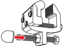
**5 Alt. c.** Slide the stand-off bumper onto the bolt.
