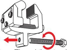
**5 Alt. a.** Thread the stand-off bolt into the lower flange of the clamp.
