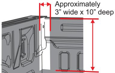
Also ensure that protrusions or logos in the drop-in liner do not interfere with the cover's operation.
