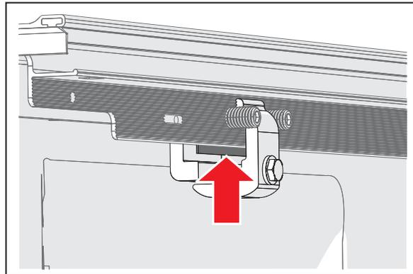
Position the clamps between the adjustment screws. Using a 9/16" or 1/2" wrench (depending on your clamps), tighten the clamps. It is important to push down on the rail while tightening, AND to tilt the rail up approximately 2 degrees simultaneously. Both the pushing down and tilting of the rail will position the rail best to minimize water intrusion.
