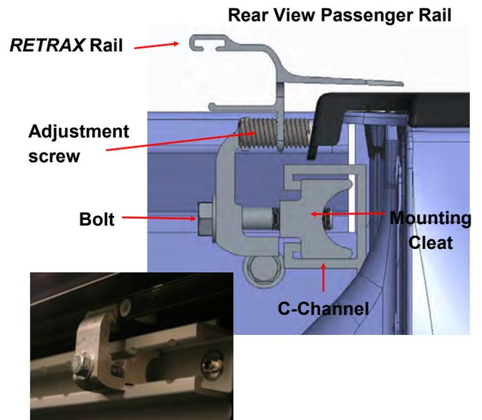
**FOR TITAN 5.5' BED:** All rail spacer screws will need to be turned approx. 5 full turns. The final spacer depth should be 0.750" from the back of the rail leg to the surface of the spacer screw that touches the truck.
