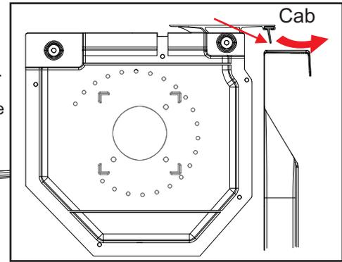
NOTE: With the cover in place, the front seal lays flat on the bulkhead, but must not extend past the bed rail cap. Trim the seal as needed to ensure that it lays flat.
