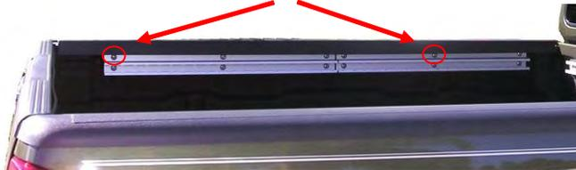
Attach all 4 rail brackets to these holes using the 4 bracket bolts (long leg points up).
