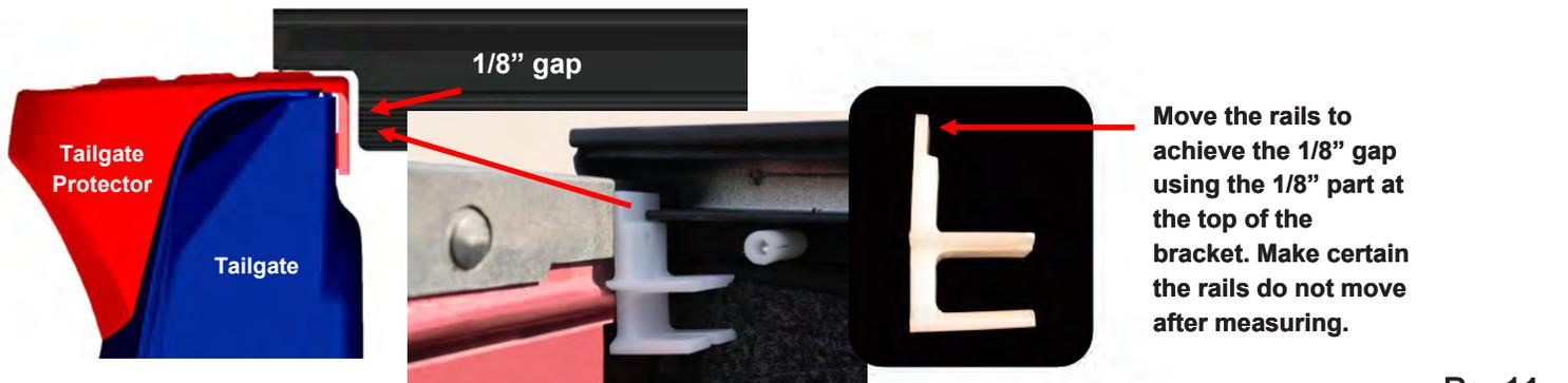
Move the rails to achieve the 1/8" gap using the 1/8" part at the top of the bracket. Make certain the rails do not move after measuring.
