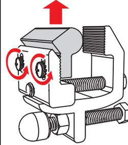
Re-tighten screws and fully engage the lock washers. Always make sure the two sets of teeth are fully engaged.
