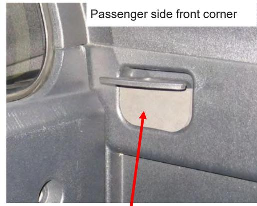
Remove the adhesive backing paper from the foam fillers for the tie-downs. Push into place over the tie-down bolts. Repeat on driver's side.
