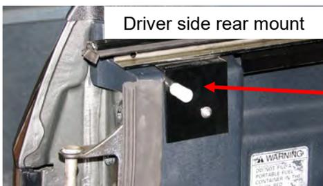
Start rear mounting screws. Slide a flat washer onto the (2) M6 x 40mm (metric) rear mount bolts, insert bolts through holes in rear rail brackets, then insert nylon spacer and start threading into factory holes at rear. Use 4mm Allen wrench.
