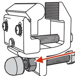
**NOTE:** if the clamps need to be removed after the stand-off bolts are set, the jam nut and bolt will have to be loosened.
