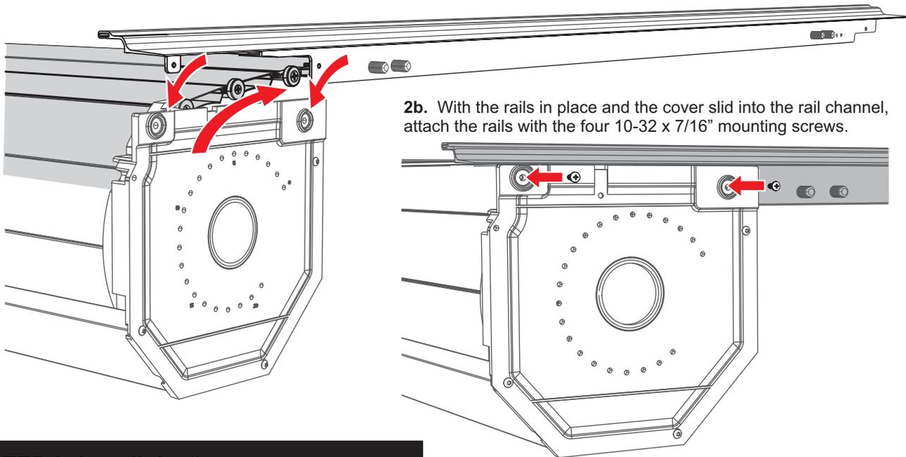
**2b.** With the rails in place and the cover slid into the rail channel, attach the rails with the four 10-32 x 7/16" mounting screws.
