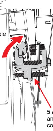
**5 Atl. f.** If the jaw does not contact firmly into the corner of the bed flange, remove the clamp and loosen the screws to adjust the jaw.
