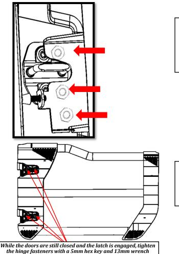
Next, close the door and align the latch on the vehicle striker pin. Push the door onto the striker until the latch fully engages with two clicks. The latch that is equipped with your tube doors are two stage latches; please make sure that both stages are engaging before proceeding.
