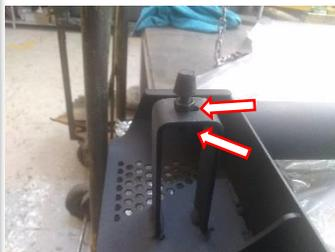
Adjust the door stop out until the rubber end firmly makes contact with the body of the vehicle. Tighten both the jam nuts with a 10mm wrench. Depending on your adjustment the jam nuts may be on opposite sides of the bracket as shown or both nuts may be installed on the inside of the bracket to provide proper clearance
