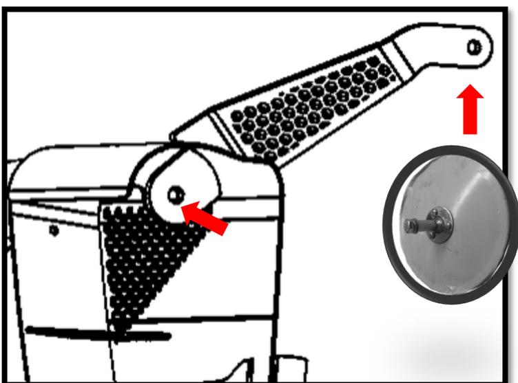
Install mirror onto the mirror bracket. Use the preassembled hardware that came with each mirror (5/16" flat washer, 5/16" lock washer, and 5/16" x 3/4" bolt). Repeat process for both sides.
