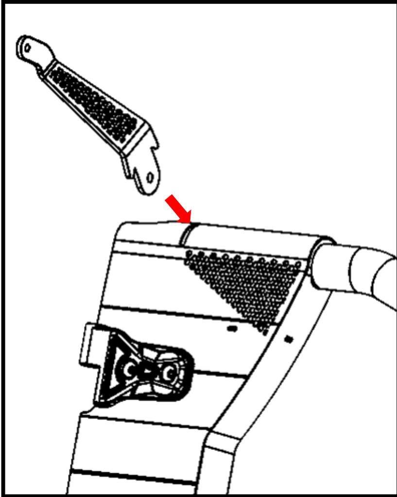
Install mirror bracket onto front door. Insert the bracket into the slot located on the top side and match it with the hole bracket located on the inside of the door. Fasten down using 3/8" x 1" hex bolt, 3/8" flat washer, 3/8" lock washer and 3/8" nut. Repeat process for both sides.
