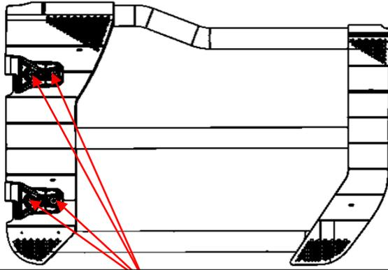
If the latch is not engaging properly you may need to loosen the latch with a 13mm wrench and a T40 torx bit. Adjust the position of the latch as needed. Tighten all fasteners after the adjustment is complete.
