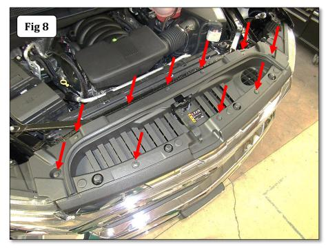
**Step-8** Using a 10mm socket and ratchet, remove the (4) screws (2) per side securing the top of the grille, (Fig 9). Working from side to side, gently pull outward on the grille to unsnap the clips by the head lights, and from the sides and center of the grille. Remove the grille from the vehicle.
