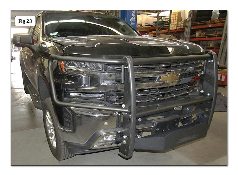
**Step-19** Attach the driver side headlight protector (not shown) to the brush guard using (1)  $\frac{14''}{4''}$  s  $\frac{34''}{4''}$  button head bolt, and the opposite end to the side plate using (2)  $\frac{5}{16''}$  x  $\frac{1''}{1''}$  button head bolts, (2)  $\frac{5}{16''}$  flat washers and (2)  $\frac{5}{16''}$  lock nuts. Repeat for the passenger side headlight protector. Align the grille and brush guard assembly, and tighten all nuts and bolts.
