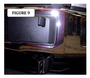
**Step-9** Place the Grille Guard over the brackets. Secure the lower brackets using (2)  $1/2 \ge 1/2$ " hex bolts, (4) 1/2" flat washers, (2) 1/2" lock washers and (2) 1/2" hex nuts. Secure to auxiliary bracket using (1)  $3/8 \ge 1 \cdot 1/4$ " hex bolt, (1) 3/8" flat washer, (1) 3/8" lock washer and (1) 3/8" hex nut. Leave loose. Figure 10.
