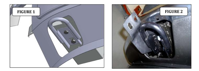
**Step-3** Slide the main bracket between the rear's tow hook bolt and frame then re-install the tow hook over the main bracket. Re-attach using the factory bolts removed in previous step. Figure 2. Leave loose. Follow to step 8.
