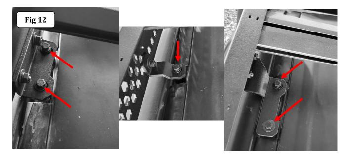
$\textbf{Step-10} \ \text{Adjust and align the SRM300 roof rack assembly as necessary and fully tighten all hardware.}$
