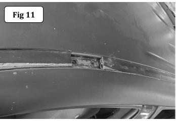
**Step-11** Cut the roof molding trim at marked areas. Install back the top molding trim and place the spacers over the holes (Fig 11).
