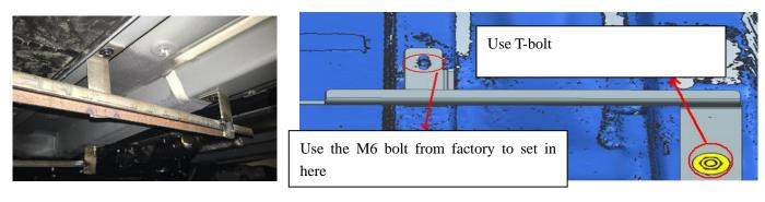
Step 5: Remove the plastic plug from vehicle bottom and then place the T-bolt to factory hole as bellow photo shown to connect the rear mounting guard (L). Finished then fasten lightly with nuts.
