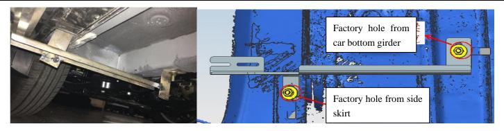
Step 4: Remove the plastic plug from vehicle bottom and then place the T-bolt to factory hole from car bottom girder as bellow photo shown to connect the center mounting guard (L). Finished then fasten lightly with nuts.
