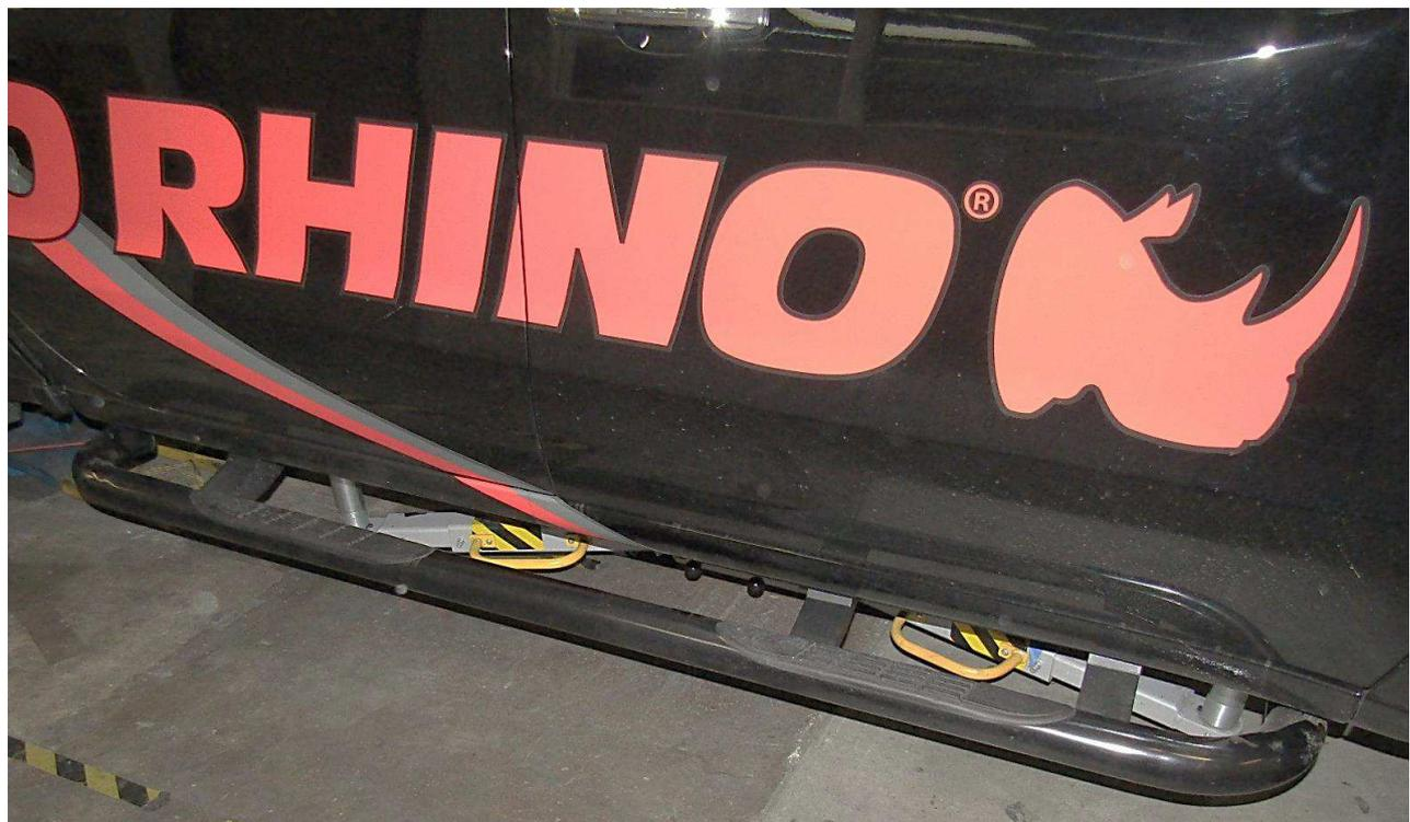
6. Repeat the installation steps to install the mounting brackets and step on the driver side. Remember to check and retighten all nuts and bolts periodically.
