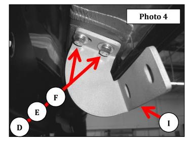
**Step-4** Attach the passenger side center and rear brackets to the body panel using (2) M8 hex bolts, (2) 5/16" lock washers and (2) 5/16" flat washers. Leave the nut and bolts loose for final adjustment, (Photo 4).
