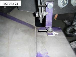
**Step-18** Secure the auxiliary side bracket to the frame using the bumper shell using (1)  $\frac{1}{2}$  x 3  $\frac{1}{2}$ " hex head bolt previously installed. Attach the opposite side end of the auxiliary side bracket to the bumper shell bracket using (1)  $\frac{1}{2}$  x 1  $\frac{1}{2}$ " hex head bolt, (2)  $\frac{1}{2}$ " flat washer, (1)  $\frac{1}{2}$ " lock washer, and (1)  $\frac{1}{2}$ " hex nut. (PICTURE 25 & 26).
