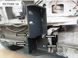
**Step-11** Position the auxiliary bracket in the frame. Secure the brackets using (3)  $\frac{1}{2}$  x 3  $\frac{1}{2}$ " hex head bolt, (4)  $\frac{1}{2}$ " flat washer, (3)  $\frac{1}{2}$ " lock washer, (1)  $\frac{1}{4}$ " spacer, near main bracket, and (3)  $\frac{1}{2}$ " hex nut. **(PICTURE 15 & 16).**
