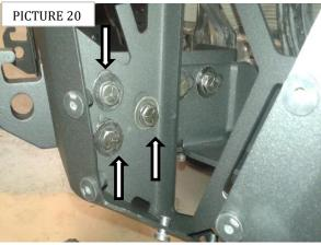
**Step-15** Secure the rear auxiliary bracket to the frame using  $\frac{1}{2} \times 3 \frac{1}{2}$ " hex head bolt previously installed. And secure the rear auxiliary bracket to the main bracket using (1)  $\frac{1}{2} \times 1 \frac{1}{2}$ " hex head bolt, (1)  $\frac{1}{2}$ " flat washer, (1)  $\frac{1}{2}$ " lock washer, and (1)  $\frac{1}{2}$ " hex nut. (**PICTURE 21 & 22**).
