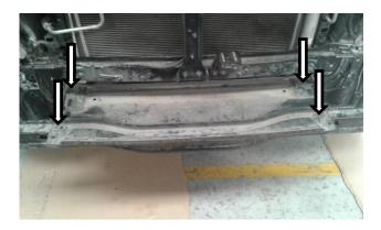
**Step-9** Locate the plastic side protectors and remove them, driver side and passenger side. ( They will no longer be used ). **(PICTURE 11).** Locate screws that secure the bumper support ( 2 ) per side and remove them. **(PICTURE 12)**
