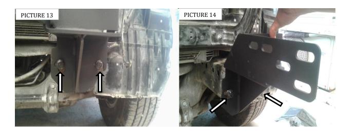
**Step-11** Position the auxiliary bracket in the frame. Secure the brackets using (1)  $\frac{1}{2}$  x 4" hex head bolt, (2)  $\frac{1}{2}$ " flat washer, (1)  $\frac{1}{2}$ " lock washer, (1)  $\frac{1}{4}$ " and (1)  $\frac{1}{2}$ " hex nut. (1)  $\frac{7}{16}$ " x 4" hex head bolt, (2)  $\frac{7}{16}$ " flat washer, (1)  $\frac{7}{16}$ " lock washer, (1)  $\frac{7}{16}$ " hex nut. (PICTURE 15 & 16).
