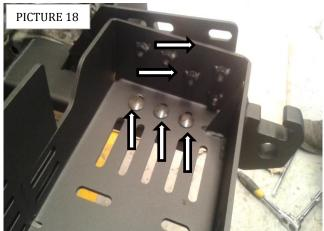
**Step-13** Adjust the mounting plate / Winch tray and brackets to the forward position, center and level the mounting plate / Winch tray with the vehicle frame then tighten all factory hex nuts and supplied nuts and bolts securing the mounting plate / Winch tray and frame brackets. Do not install the fairlead at this time.
