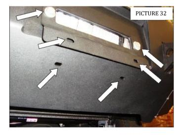
**Step-25** If installing a winch, attach the license plate directly to the (2) obround holes in the lower face of the bumper shell using the supplied 1/4" bolts and nuts. ( **PICTURE 32**).
