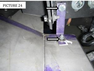
**Step-17** Secure the auxiliary side bracket to the frame using the bumper shell using (1)  $\frac{1}{2}$  x 3  $\frac{1}{2}$ " hex head bolt previously installed. Attach the opposite side end of the auxiliary side bracket to the bumper shell bracket using (1)  $\frac{1}{2}$  x 1  $\frac{1}{2}$ " hex head bolt, (2)  $\frac{1}{2}$ " flat washer, (1)  $\frac{1}{2}$ " lock washer, and (1)  $\frac{1}{2}$ " hex nut. (PICTURE 25 & 26).
