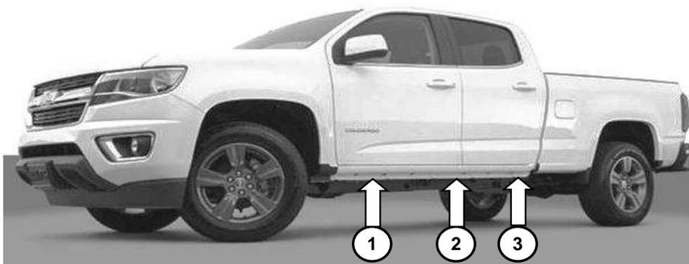
1. Begin the installation on the driver side. Starting at the front of the vehicle, locate and remove the plastic plugs in the back side and bottom of rocker panel to expose the holes used for placement of the 5/16" Clip- Nuts, **(Photo 2)**.
