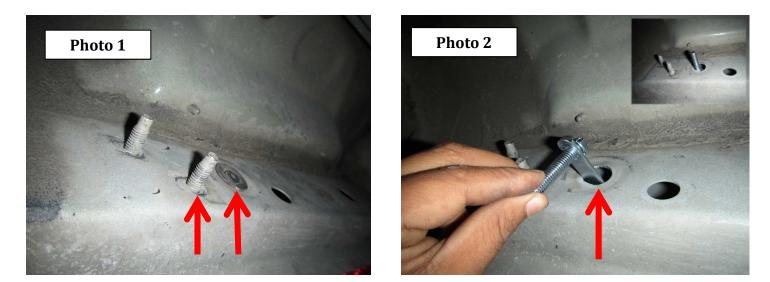
**Step-2** Attach one of the driver side brackets to the rocker panel using the (1) M8 Flange nut to the existing bolt, and (1)5/16" hex nut, (1) 5/16" lock washer and (1) 5/16" flat washer to the bolt plate. Leave the nut and bolts loose for final adjustment. **(Photo 3)**.
