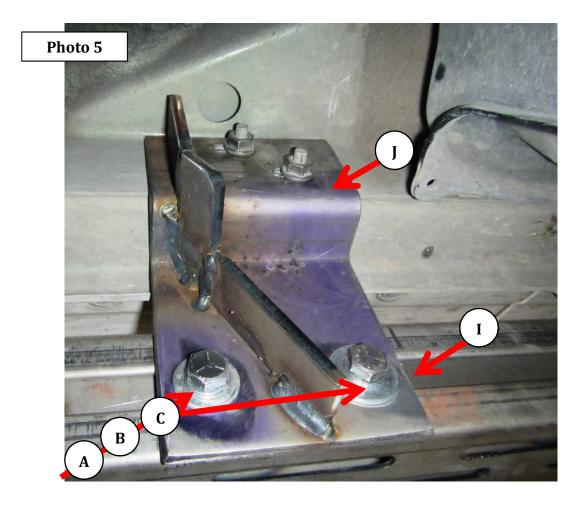
**Step-5** Align the Dominator D6 with the vehicle and tighten all bracket and side step nuts and bolts,. Repeat the above steps to install the passenger side brackets and running board. Remember to check and retighten the nuts and bolts every six months.
