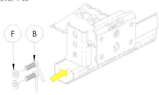
Install a ½" flat washer onto the supplied ½" bolt rods.
