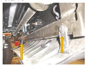
• Remove the 2 plastic pushpins securing the rear of the air dam to the frame cross member.
