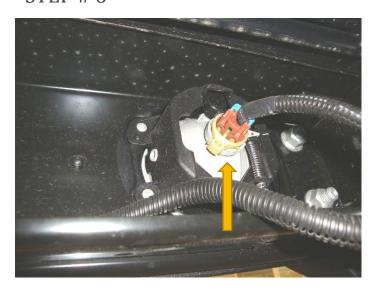
• If equipped, disconnect the wiring harness from the fog lights.
