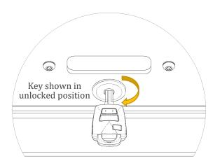
STEP# 20.4 Key is now in unlocked position. Rotate 90° clockwise to lock.
