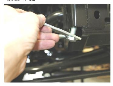
• Insert one of the supplied ½" bolt plates through frame opening as shown.
