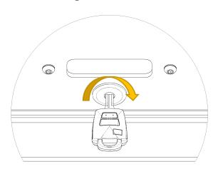
STEP# 20.3 While maintaining FULL key insertion, rotate key clockwise until it hits a stop point at about 3/4 of a turn or 270 degrees.
