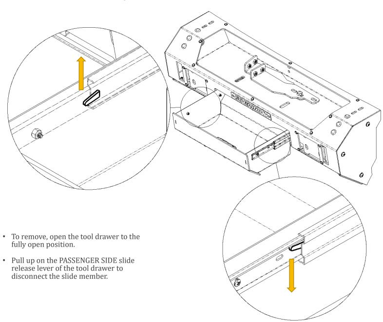
Press down on the DRIVER SIDE slide release lever of the tool drawer to disconnect the slide member. Once both sides are disconnected pull the tool drawer forward and remove it.
