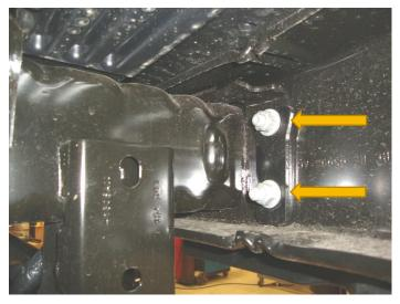
• Remove the 4 nuts from the studs securing the factory bumper to the frame using an 18mm socket. Both sides.
