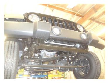
Remove the air dam from the underside of the vehicle.
