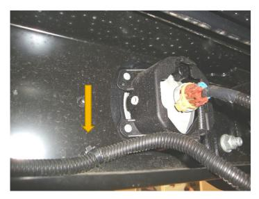
• Unclip the cable ties securing the wiring harness to the bumper.
