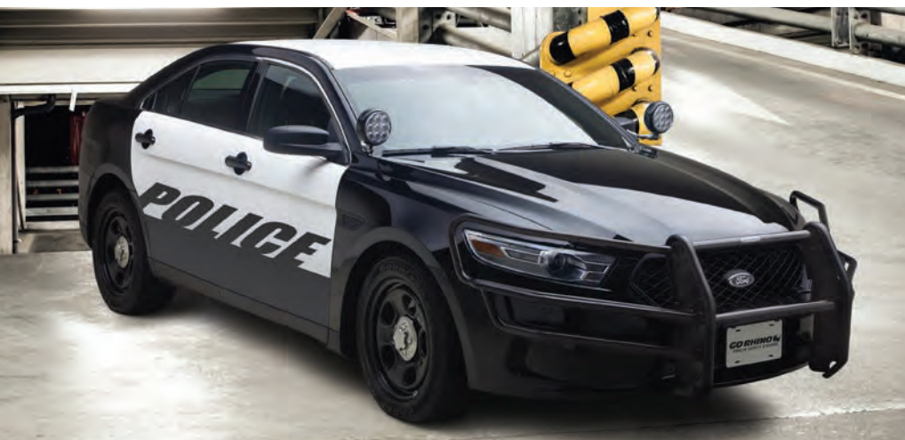
PUSH BUMPER WITH HEAVY DUTY WRAPAROUND BRUSH GUARDS
