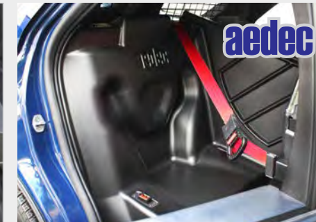
Virtually indestructible TPO seat's indentation for handcuffed detainee.
