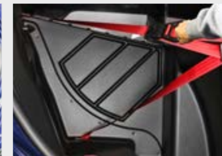
3-Point Pro-strait Harness prevents need to reach across the detainee when buckling.
