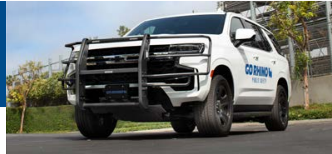
PUSH BUMPER WITH HEAVY DUTY WRAPAROUND BRUSH GUARDS
