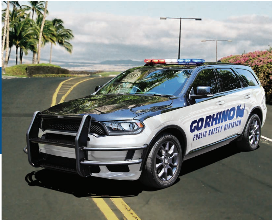
PUSH BUMPER WITH LOWER HD WRAP
