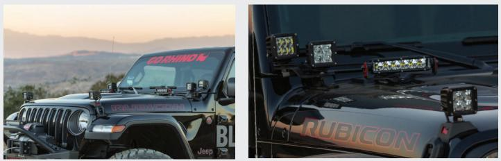
Light mounts allow for installation of lights to the hood hinge, lower A-pillar, the upper cowl, hood clamp, or hard top.
